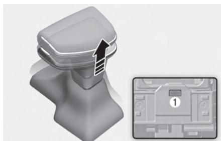
1. Pull the boot on the shift lever to remove it from the console.
