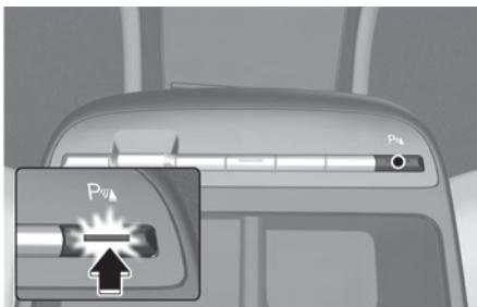
Press the Parking Safety (P $\uparrow$ ) button to turn on Forward/Reverse Parking Distance Warning. Press the button again to turn off the function.
