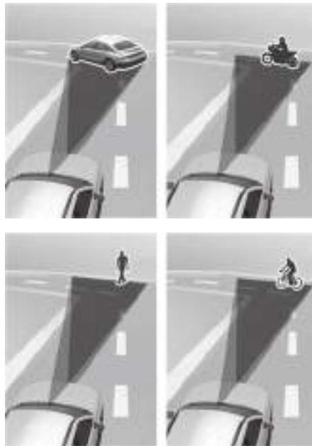
Forward Collision-Avoidance Assist may detect a vehicle, powered two-wheeler, pedestrian or cyclist in the next lane or outside the lane when driving on a curved road.
