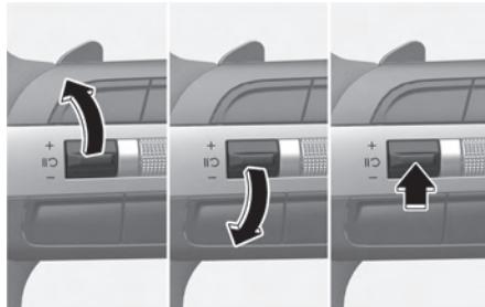
To resume Manual Speed Limit Assist after the function was paused, operate the **+, -**, **CII** switch.
