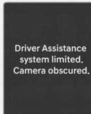
When the front windshield where the front view camera is located is covered with foreign material, such as snow or rain, it can reduce the detecting performance and temporarily limit or disable Intelligent Speed Limit Assist. If this occurs, the "**Driver Assistance system limited. Camera obscured.**" warning message and (✉) warning light will appear on the instrument cluster.
