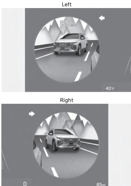
Blind-Spot View Monitor uses the wide-side view cameras to display the rear blind spot areas of your vehicle on the instrument cluster when the turn signal is turned on to help with safe lane changes.
