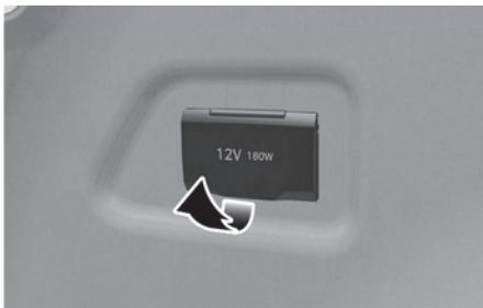
The power outlet is designed to provide power for mobile phones or other devices designed to operate with vehicle electrical systems. The devices should draw less than 12 V, 180 W with the engine running.
