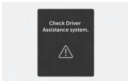
When Rear Cross-Traffic Collision-Avoidance Assist is not working properly, the "**Check Driver Assistance system.**" warning message appears on the instrument cluster for several seconds, and the master (⚠) warning light illuminates on the instrument cluster. If this occur, have vehicle inspected by an authorized HYUNDAI dealer.
