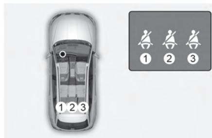
As a reminder to the rear passenger, the rear passenger's seat belt warning lights will illuminate for about 6 seconds each time the Engine Start/Stop button is in the ON position regardless of belt fastening.
