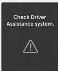
When Blind-Spot Collision-Avoidance Assist is not working properly, the "**Check Driver Assistance system.**" warning message will appear on the instrument cluster for several seconds, and the master (Δ) warning light will appear on the instrument cluster. If this occurs, have your vehicle inspected by an authorized HYUNDAI dealer.
