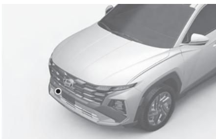
The front radar is mounted behind the front grill.
