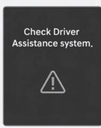
When Safe Exit Warning is not working properly, the "**Check Driver Assistance system.**" warning message will appear on the instrument cluster for several seconds, and the master warning light (⚠) will appear on the instrument cluster. If this occurs, have your vehicle inspected by an authorized HYUNDAI dealer.
