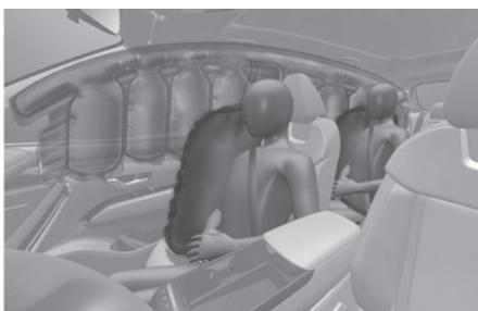
The side airbags are designed to deploy during certain side impact collisions, depending on the crash severity.
