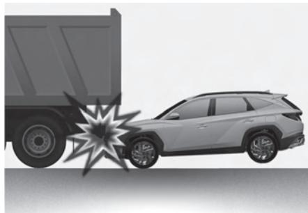
Just before impact, drivers often brake heavily. Such heavy braking lowers the front portion of the vehicle causing it to "nosedive". This is particularly important when the vehicle in front has a higher ground clearance. Airbags may not inflate if your vehicle is in a "nosedive" condition because the collision forces detected by the sensors may have been significantly reduced.
