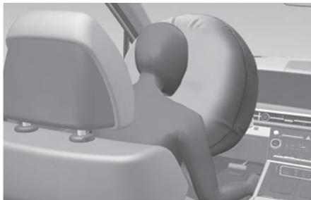
Upon deployment, tear seam in the pad cover separates from the expansion of the airbags.
