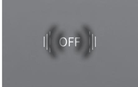
Press the **OFF** button to turn off the climate control system. You can still operate the mode buttons and air intake buttons as long as the Engine Start/Stop button is in the ON position.
