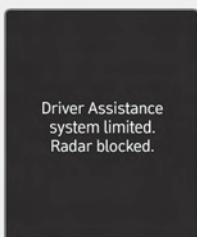
When the rear bumper around the rear-side radar or sensor is covered with foreign material, such as snow or rain, or installing a trailer or carrier, it can reduce the detecting performance and temporarily limit or disable Rear Cross-Traffic Collision-Avoidance Assist. If this occurs, the "**Driver Assistance system limited. Radar blocked.**" warning message appears on the instrument cluster.
