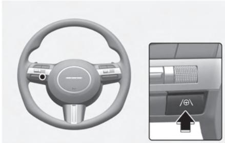
With the engine on, shortly press the Lane Driving Assist button located on the steering wheel to turn on Lane Following Assist. The gray or green (Θ) indicator light will illuminate on the instrument cluster.
