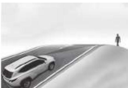
Forward Collision-Avoidance Assist may not detect other vehicles, powered two-wheeler, pedestrians or cyclists in front of you while driving uphill or downhill, adversely affecting the performance of the sensors.
