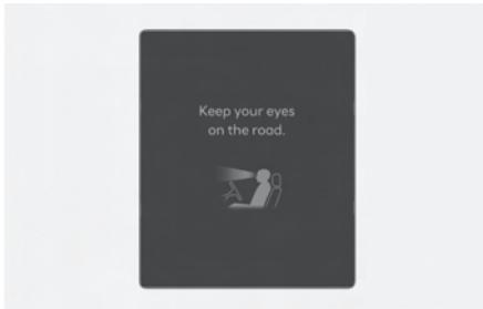
Forward Attention Warning determines whether the driver is focused on the road depending on information, such as the amount of time the driver is looking elsewhere, the amount of time the eyes are closed, how frequently the driver yawns, etc. If Forward Attention Warning judges the driver is not focused, the '**Keep your eyes on the road.**' warning message will appear on the cluster, and an audible warning will sound.
