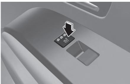
While the engine is running, press the button to warm the driver's seat or front passenger's seat.
