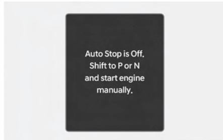
When the system is deactivated, the ISG off button indicator illuminates and a message appears on the cluster display with a warning sound if:
