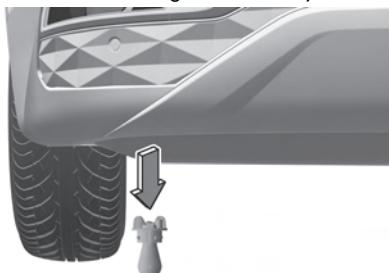
2. Loosen the retaining clips under the bumper and screws on the wheel house trim.
