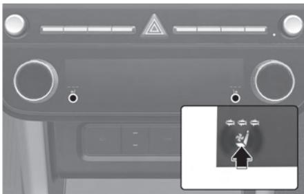
While the engine is running, press the button to cool the driver's seat or front passenger's seat.
