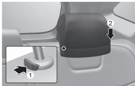
To reinstall the head restraint:
