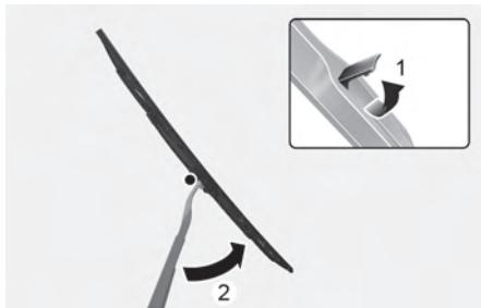
3. Lift up the wiper blade clip (1). Then pull down the wiper blade (2).
