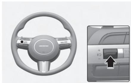
Press the **CII** switch to temporarily pause the set speed limit. The set speed limit will turn off but the Speed Limit (**CII LIMIT**) indicator will stay on.
