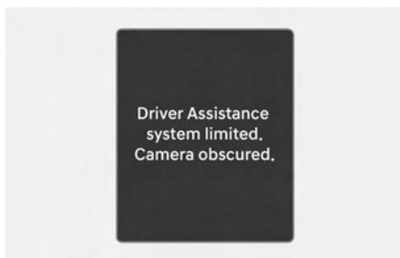
When the front windshield where the front view camera is located is covered with foreign material, such as snow or rain, it can reduce the detecting performance and temporarily limit or disable Driver Attention Warning.
