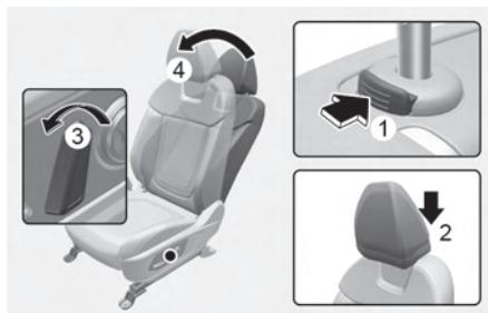
To remove the head restraint:
