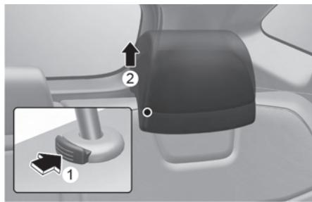
To remove the head restraint:
