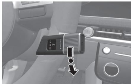
To shift the gear R (Reverse), rotate the rotary gear shift dial to R (Reverse) while depressing the brake pedal.
