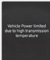
If you continue to drive with overheated transmission, the above warning message appears and self-protection mode restricts the power output of the vehicle.
