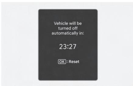
When all the conditions are satisfied, the Vehicle Auto-Shut Off operates and turns the engine off automatically after 60 minutes.
