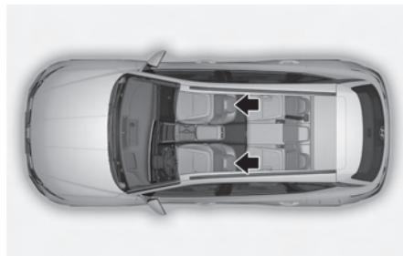
The driver's and front passenger's seats are equipped with adjustable head restraint for the passengers safety and comfort.
