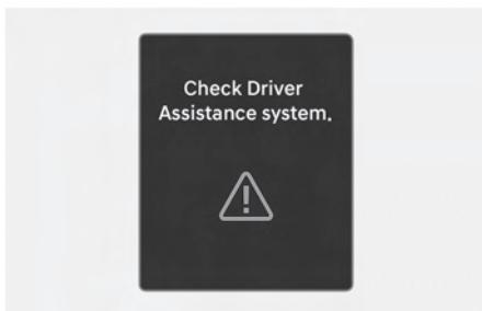
When Driver Attention Warning is not working properly, the "**Check Driver Assistance system**" warning message will appear on the cluster for several seconds, and the master (Δ) warning light and the inattentive driving (₩) warning light will appear on the instrument cluster. If this occurs, have your vehicle inspected by an authorized HYUNDAI dealer.
