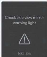
When the side view mirror warning light is not working properly, the "**Check side view mirror warning light**" warning message appears on the instrument cluster for several seconds, and the master (⚠) warning light illuminates on the instrument cluster. If this occur, have your vehicle inspected by an authorized HYUNDAI dealer.
