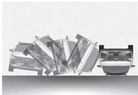
Front airbags may not inflate in rollover crash because front airbag deployment would not provide additional occupant protection.
