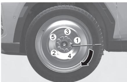
12. Use the wheel lug wrench to tighten the lug nuts in the order shown. Double-check each lug nuts until they are tight. After changing tires, have the vehicle inspected by an authorized HYUNDAI dealer tighten the lug nuts to their proper torque as soon as possible. The lug nut should be tightened to 79-94 lbf. ft (11-13 kgf.m).
