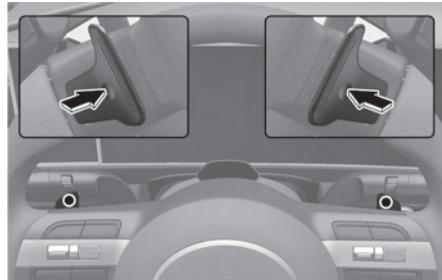
The paddle shifter is available when the shift lever/dial is in the D (Drive) position or the manual shift mode.
