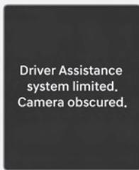
When the front windshield where the front view camera is located or the sensor is covered with foreign material, such as snow or rain, it can reduce the detecting performance and temporarily limit or disable Forward Collision-Avoidance Assist.
