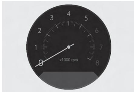
The tachometer indicates the approximate number of engine revolutions per minute (RPM). Use the tachometer to select the correct shift points and to help prevent luggering and/or over-revving the engine.
