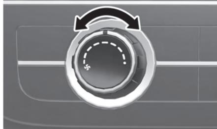
Turn the knob to the right to increase the fan speed and airflow. Turn the knob to the left to decrease fan speed and airflow. Setting the fan speed control knob to the "0" position turns off the fan.
