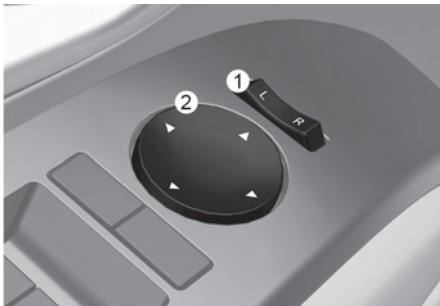
1. Press the switch (1) either to the L (left side) or R (right side) to select the side view mirror you want to adjust.
