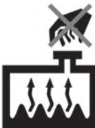
Never remove the engine coolant reservoir cap or the drain plug while the engine and radiator are hot. Hot coolant and steam may blow out under pressure, causing serious injury.
