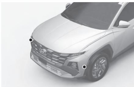
These ultrasonic sensors are mounted near the front wheels outside your vehicle.
