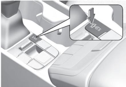
Press the ISG OFF button to turn off the ISG system. The ISG OFF button indicator illuminates. To use the system, press the ISG OFF button again.
