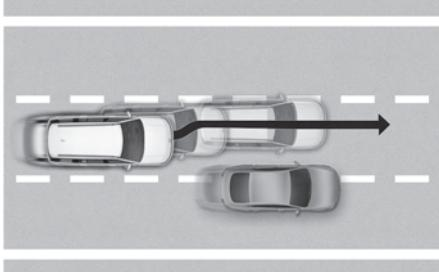
When vehicle speed is above 40 mph (60 km/h), if a vehicle around you is driving at a close distance, your vehicle will control steering in the opposite direction of the vehicle to assist in safe driving.
