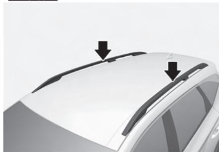
Your vehicle may come equipped with roof side rails. If your vehicle is equipped with roof side rails, you can add roof rack crossbars as an accessory (not shown).
