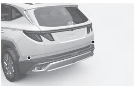
The rear corner radars are mounted near the rear corners of your vehicle above the bumper.
