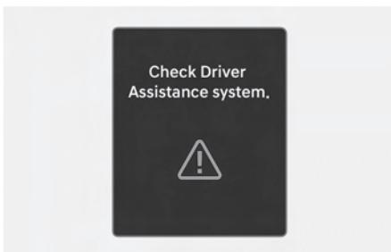
When High Beam Assist is not working properly, the '**Check Driver Assistance system**' warning message may appear, and the (AUTO) warning light may illuminate on the instrument cluster. Contact an authorized HYUNDAI dealer.
