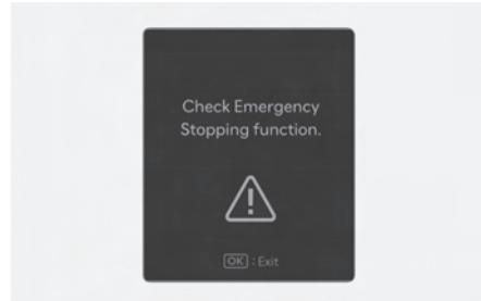
When Emergency Stop is not working properly, the "Check Emergency Stopping function." warning message appears, and the master (Δ) warning light illuminates on the instrument cluster. If this occurs, have your vehicle inspected by an authorized HYUNDAI dealer.
