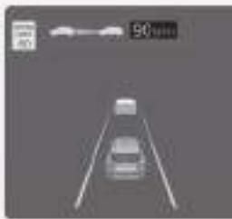
When driving at a speed higher than the displayed speed limit, the speed limit is displayed in red.
