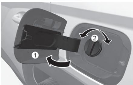
5. To remove the fuel tank cap (2), turn it counterclockwise. A hissing noise is heard because the pressure inside the tank equalizes.
