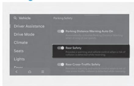
With the engine on, select or deselect **Setup > Vehicle > Driver Assistance > Parking Safety** in the infotainment system to set whether to use each function.
