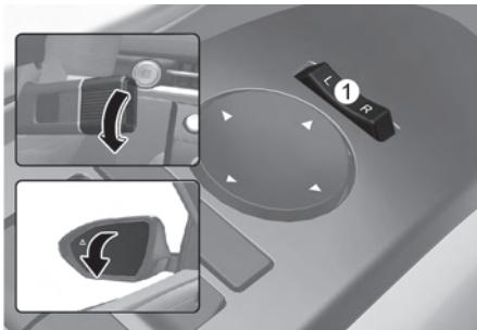
When the gear is shifted to the R (Reverse) position, the side view mirrors rotate downwards to aid with driving in reverse.
