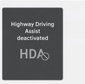
If the driver still does not have their hands on the steering wheel after the hands-off warning, **"Highway Driving Assist deactivated"** warning message will appear and Highway Driving Assist will be automatically canceled.
