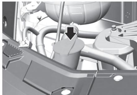
Check the fluid level in the washer fluid reservoir and add fluid if necessary. Plain water can be used during summer months if washer fluid is not available. However, use washer fluid with antifreeze in cold climates to prevent freezing.
