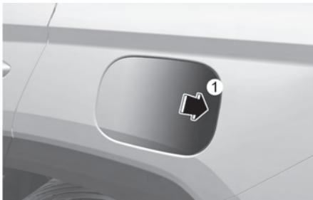
4. Pull the fuel filler door outward to access the fuel tank cap (2).
