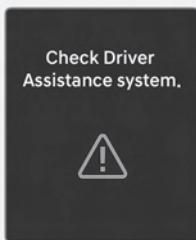
When Forward Collision-Avoidance Assist is not working properly, the "**Check Driver Assistance system.**" warning message will appear, and the (Δ) or (✖) warning lights will illuminate on the cluster display. Have the vehicle inspected by an authorized HYUNDAI dealer.
