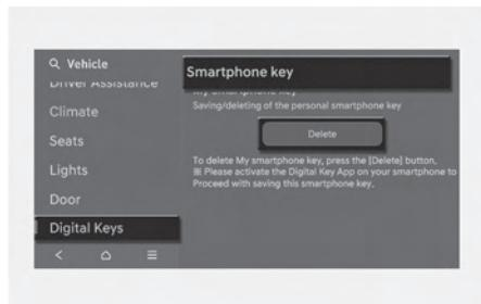
To delete only my registered digital key (smartphone), select **Setup > Vehicle > Digital Keys > Smartphone key > My Smartphone Key > Delete** from the infotainment system.
