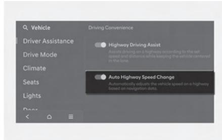
With the engine on, select **Setup > Vehicle > Driver Assistance > Driving Convenience > Auto Highway Speed Change** from the infotainment system to turn on Navigation based Smart Cruise Control and deselect to turn off the function.
