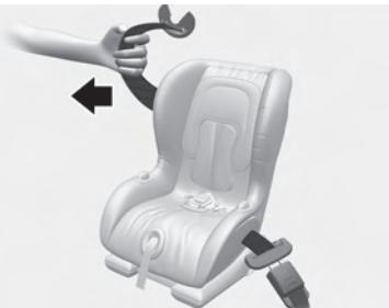
4. Slowly allow the shoulder portion of the seat belt to retract and listen for an audible "clicking" or "ratcheting" sound. This indicates that the retractor is in the Automatic Locking mode. If no distinct sound is heard, repeat Step 3 and 4.
