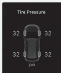
The tire pressure of each tire appears. For more information, refer to the "Tire Pressure Monitoring System (TPMS)" section in chapter 8.
