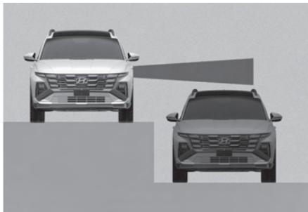
Blind-Spot Collision-Avoidance Assist may not operate properly when driving where the heights of the lanes are different. The function may not detect the vehicle on a road with different lane heights (underpass joining section, grade separated intersections, etc.).
