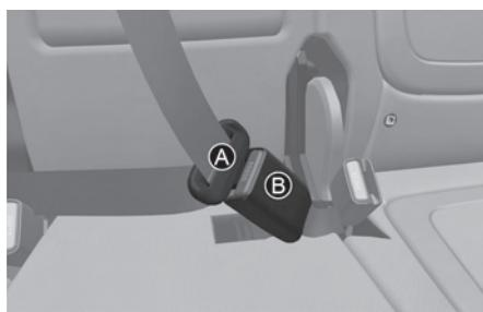
Insert the tongue plate (A) into the buckle (B) until an audible "click" is heard, indicating the latch is locked. Pull the shoulder portion of the belt to snug the belt across your hips and remove slack. Make sure the seat belt is not twisted.
