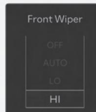
This indicator displays which wiper speed is selected using the wiper control.
