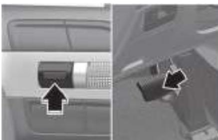
Press the **SCC** switch or depress the brake pedal to temporarily cancel Smart Cruise Control.
