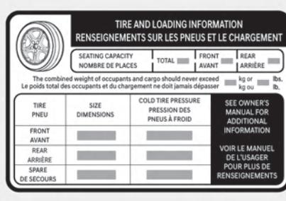
The label located on the driver's door jamb shows the original tire size, cold tire pressures recommended for your vehicle, the number of people that can be in your vehicle and vehicle capacity weight.
