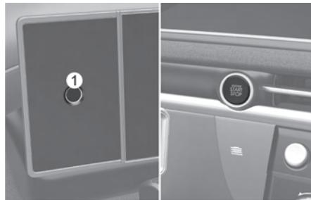
Place your finger on the fingerprint sensor (1) to verify your fingerprint. After it is successfully verified, start the engine by pressing the Engine Start/Stop button within 30 seconds.
