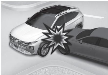
Front airbags may not inflate in side impact collisions, because occupants move in the direction of the collision.
