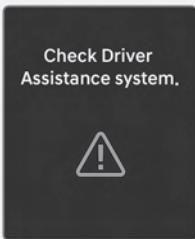
When Highway Driving Assist is not working properly, the "**Check Driver Assistance system.**" warning message and yellow Lane Keeping Assist (/ $\backslash$ ) warning light appears on the instrument cluster. If this occurs, have your vehicle inspected by an authorized HYUNDAI dealer.
