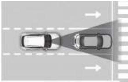
Forward Collision-Avoidance Assist is designed to help detect and monitor the vehicle ahead or help detect a powered two-wheeler, pedestrian or cyclist in the roadway and warn the driver that a collision is imminent with a warning message and warning and apply emergency braking.
