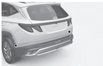
These ultrasonic sensors are mounted near the rear wheels outside your vehicle.
