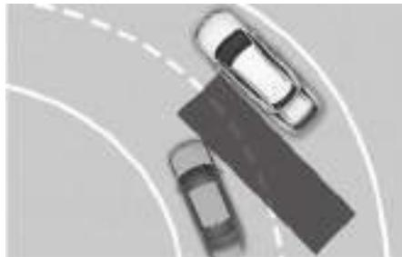
Blind-Spot Collision-Avoidance Assist may not operate properly when driving on a curved road. The function may not detect the vehicle in the next lane.
