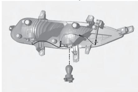
4. Remove the socket from the assembly by turning the socket counterclockwise until the tabs on the socket align with the slots on the assembly.
