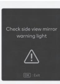
When the side view mirror warning light is not working properly, the "**Check side view mirror warning light**" warning message will appear on the instrument cluster for several seconds, and the master (Δ) warning light will illuminate on the instrument cluster. If this occurs, have your vehicle inspected by an authorized HYUNDAI dealer.
