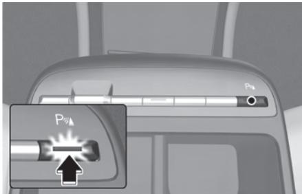
Press and hold the Parking Safety (P $\uparrow$ ) button more than 2 seconds, to turn the Parking Collision-Avoidance Assist on or off.
