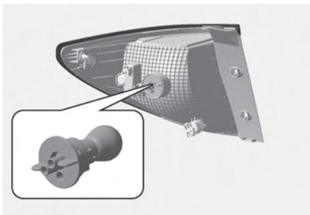
6. Remove the bulb from the socket by pressing it in and rotating it counterclockwise until the tabs on the bulb align with the slots in the socket. Pull the bulb out of the socket.
