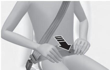
Improperly positioned seat belts may increase the risk of serious injury in a crash. Take the following precautions when adjusting the seat belt:
