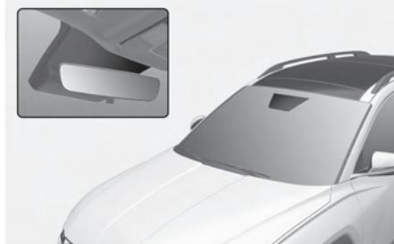
The Auto defogging reduces the possibility of fogging up the inside of the windshield by automatically sensing the moisture on inside the windshield.
