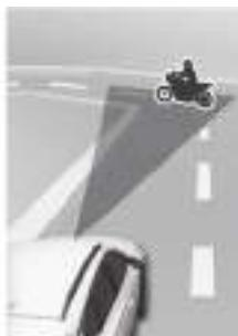
Forward Collision-Avoidance Assist may not detect other vehicles, pedestrians or cyclists in front of you when driving on curved roads adversely affecting the performance of the sensors. This may result in no warning or braking assist when necessary.
