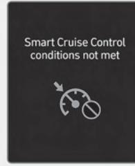
If the Driving Assist button, + switch, - switch or II $\circ$  switch is operated when Smart Cruise Control operating conditions are not satisfied, the "**Smart Cruise Ctrl. conditions not met**" will appear on the instrument cluster, and an audible warning will sound.
