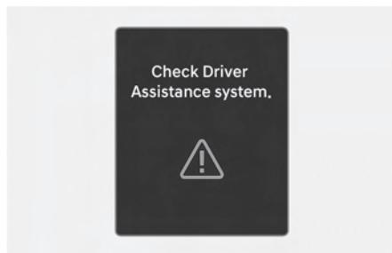
When Forward Collision-Avoidance Assist is not working properly, the "Check Driver Assistance system." warning message will appear, and the (⚠) or (⚠) warning lights will illuminate on the instrument cluster. Have your vehicle inspected by an authorized HYUNDAI dealer.
