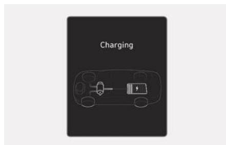
The high voltage battery is charged up by the regenerative brake system.
