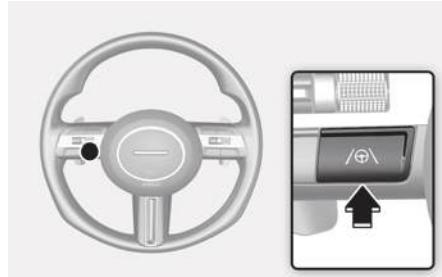
With the engine on, shortly press the Lane Driving Assist button located on the steering wheel to turn on Lane Following Assist. The gray or green (⌚) indicator light will appear on the instrument cluster.
