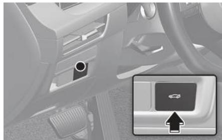
When the trunk is closed, press the power trunk open/close button. The power trunk opens with a warning sound.
