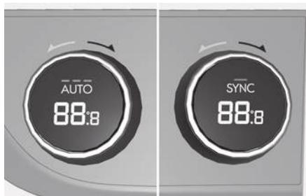
Turn right the knob to increase the temperature. Turn left the knob to decrease the temperature.
