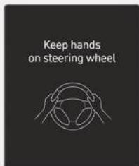
If the driver takes their hands off the steering wheel for several seconds, the **"Keep hands on steering wheel"** warning message appears on the instrument cluster, and an audible warning sounds in stages.
