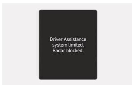
When the rear bumper around the rear-side radar or sensor is covered with foreign material, such as snow or rain, or installing a trailer or carrier, it can reduce the detecting performance and temporarily limit or disable Rear Cross-Traffic Collision-Avoidance Assist. If this occurs, the "**Driver Assistance System limited. Radar blocked.**" warning message appears on the instrument cluster.
