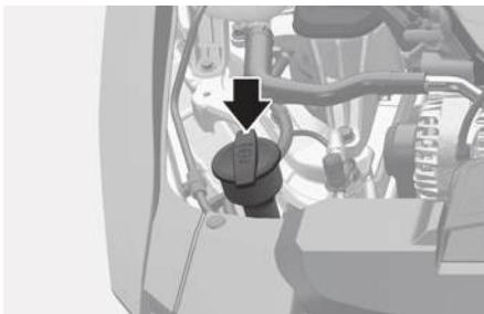
Check the fluid level in the washer fluid reservoir and add fluid if necessary. Plain water may be used if washer fluid is not available. However, use washer solvent with antifreeze characteristics in cold climates to prevent freezing.
