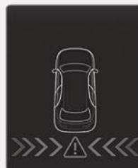
When the Rear Cross-Traffic Collision-Avoidance Assist is operating, if the function is not working normally or the radar is blocked, the master warning light (
