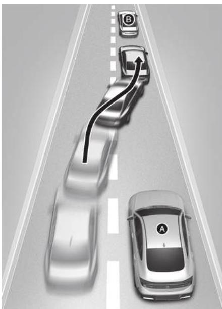
When a vehicle moves into your lane from an adjacent lane, it cannot be detected by the sensor until it is in the sensor's detection range. The smart recuperation system may not immediately detect the vehicle when your vehicle changes lanes abruptly.
