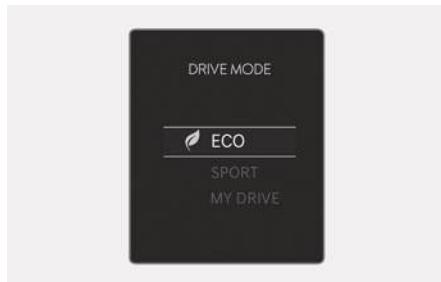
The mode changes whenever the driver pushes the DRIVE MODE switch up or down.
