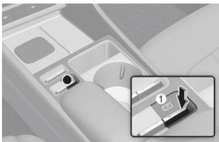
Press the Parking/View button (1) while the gear is in P (Park) to turn on the Rear View Monitor.
