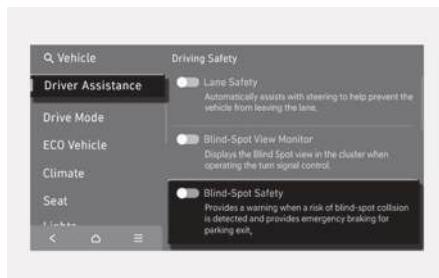
With the engine on, select **Setup > Vehicle > Driver Assistance > Driving Safety > Blind-Spot Safety** from the settings menu to set whether to use each function.
