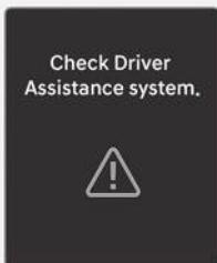
When Driver Attention Warning is not working properly, the "**Check Driver Assistance system.**" warning message will appear on the instrument cluster for several seconds, and the master (⚠) warning light and the inattentive driving (⚠) warning light will appear on the instrument cluster. If this occurs, have your vehicle inspected by an authorized HYUNDAI dealer.
