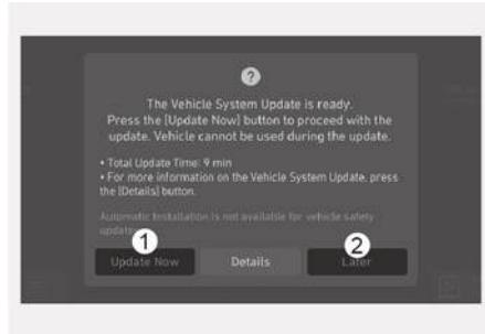
After the vehicle ignition is turned off, the vehicle system will provide the option to start the update.
