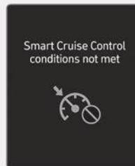
If the Driving Assist button, + switch, - switch or (II) switch is operated when Smart Cruise Control operating conditions are not satisfied, the "**Smart Cruise Control conditions not met**" will appear on the instrument cluster, and an audible warning will sound.
