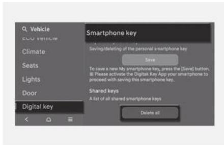
To delete all the registered digital key (smartphone), from the Settings menu select **Setup > Vehicle > Digital Keys > Smartphone key > Delete all** in the infotainment system.
