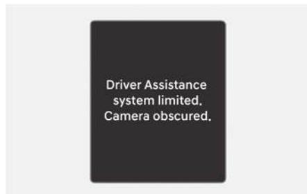
When the front windshield where the front view camera is located is covered with foreign material, such as snow or rain, it can reduce the detecting performance and temporarily limit or disable Intelligent Speed Limit Assist. If this occurs, the "**Driver Assistance system limited. Camera obscured.**" warning message and the speed limit (⊖) warning light will appear on the instrument cluster.
