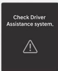
When Forward Collision-Avoidance Assist is not working properly, the "**Check Driver Assistance system.**" warning message will appear, and the (⚠), (⚠) warning light will illuminate on the instrument cluster. Have your vehicle inspected by an authorized HYUNDAI dealer.
