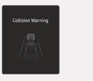
To warn the driver of a collision, the "**Collision Warning**" warning message appears and the (⚠) warning light blinks on the instrument cluster with a warning sound and the steering wheel vibrates.
