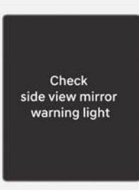
When the side view mirror warning light is not working properly, the "**Check side view mirror warning light**" warning message will appear on the instrument cluster for several seconds, and the master (⚠) warning light will appear on the instrument cluster. If this occurs, have your vehicle inspected by an authorized HYUNDAI dealer.
