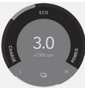
The power gauge indicates whether the current driving condition is fuel efficient or not.
