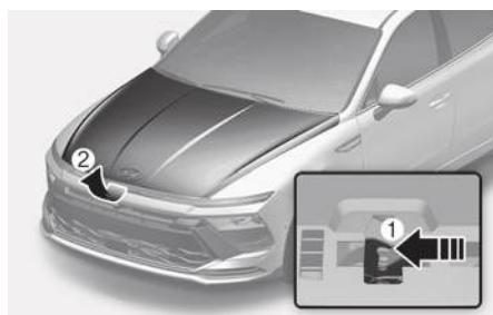
3. Go to the front of the vehicle, raise the hood slightly, push up the secondary hood release lever (1) inside of the hood center and lift the hood (2).
