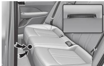
The hybrid battery cooling duct is located below the center of the rear seat. The cooling duct cools down the hybrid battery. When the hybrid battery cooling duct is blocked, the hybrid battery may be overheated.
