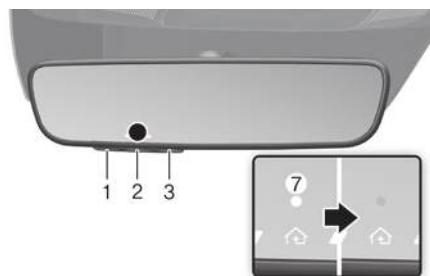
1. Press and hold the buttons (1) and (3) simultaneously
