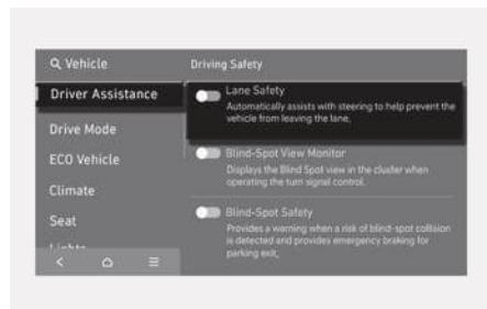
With the engine on, select **Setup > Vehicle > Driver Assistance > Driving Safety > Lane Safety** from the settings menu in the infotainment system to set whether to use each function.
