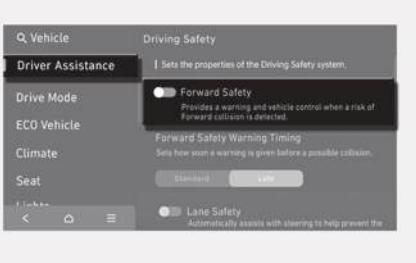
With the engine on, select **Setup > Vehicle > Driver Assistance > Driving Safety** from the settings menu in the infotainment system to set whether to use each function.
