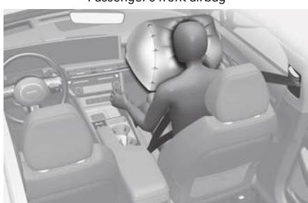
After complete inflation, the airbag immediately starts deflating, enabling the driver to maintain forward visibility and steer or operate other controls.
