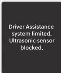
If this occurs the "**Driver assistance system limited. Ultrasonic sensor blocked**" warning message appears on the instrument cluster. Parking Distance Warning operates properly when snow, rain or foreign material is removed. If Parking Distance Warning does not operate properly after obstruction (snow, rain, or foreign material) is removed (including trailer, carrier, etc., from the rear bumper), have your vehicle inspected by an authorized HYUNDAI dealer.
