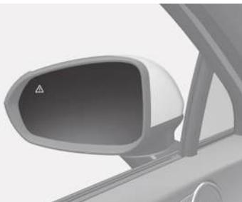
To warn the driver a vehicle is detected, the warning light on the side view mirror illuminates.
