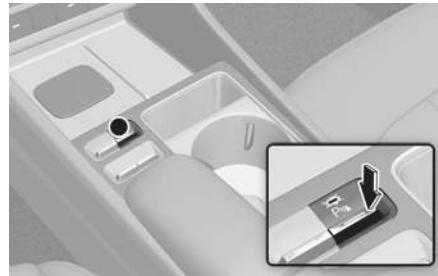
Press the Parking Safety (P $\Delta$ ) button to turn on Parking Distance Warning. Press the button again to turn off the function.
