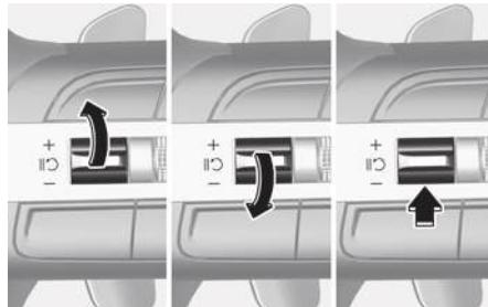
To resume Manual Speed Limit Assist after the function was paused, operate the +, -, or (II) switch.
