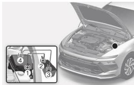
6. Connect the jumper cables in the exact sequence shown in the illustration. First connect one jumper cable to the red, positive (+) battery/jumper terminal of your vehicle (1).
