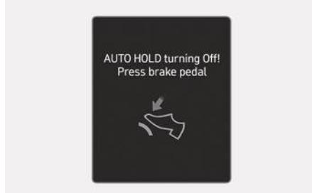
When the conversion from Auto Hold to EPB is not working properly a warning will sound and a message will appear.
