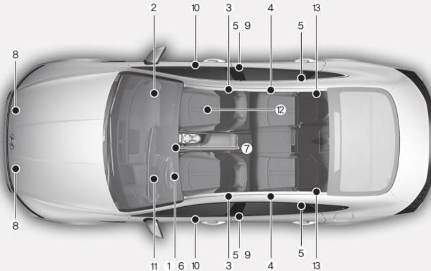
The SRS consists of the following components:
