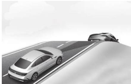
During uphill or downhill coasting, the smart recuperation system may not detect a moving vehicle in your lane, and cause your vehicle to accelerate. Also, your vehicle speed decelerates when a vehicle ahead is detected suddenly. Apply the brake pedal or accelerator pedal depending on the road and driving conditions.
