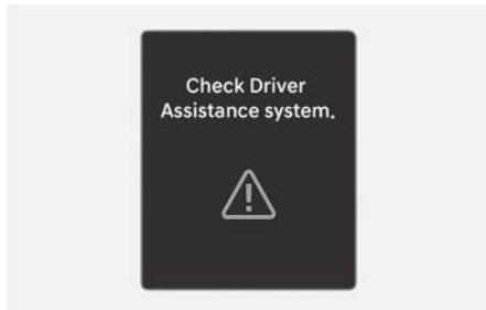
When Lane Keeping Assist is not working properly, the "**Check Driver Assistance system.**" warning message and yellow Lane Keeping Assist (/ $\Delta$ ) warning light appears on the instrument cluster. If this occurs, have your vehicle inspected by an authorized HYUNDAI dealer.
