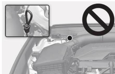
High voltage cut-off switch is a device located inside the engine compartment to block the battery's high voltage when your vehicle is inspected at an authorized HYUNDAI dealer.
