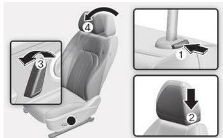
1. Recline the seat back by pressing seatback angle lever or switch (3).
