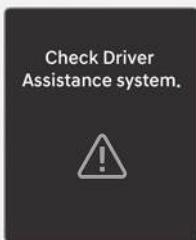
When Blind-Spot Collision-Avoidance Assist is not working properly, the "**Check Driver Assistance system.**" warning message will appear on the instrument cluster for several seconds, and the master (⚠) warning light will appear on the instrument cluster. If this occurs, have your vehicle inspected by an authorized HYUNDAI dealer.
