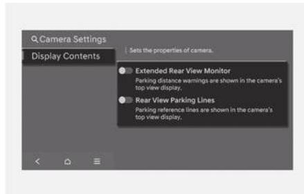
You can change Rear View Monitor **Display Contents** by touching the setup icon (⚙) on the screen while rear view Monitor is operating, or selecting **Setup > Vehicle > Driver Assistance > Parking Safety > Camera Settings** from the Settings menu in the infotainment system while the engine is on.
