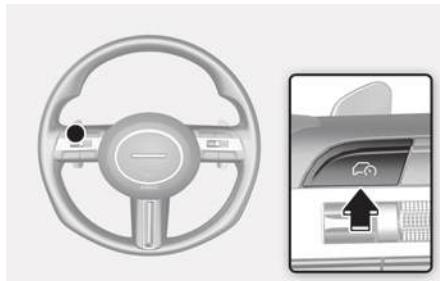
2. Push the + switch up or - switch down, and release it at the desired speed. Push the + switch up or - switch down and hold it. The speed will increase or decrease to the nearest multiple of 5 (multiple of 10 in km/h) at first, and then increase or decrease by 5 mph (10 km/h).
