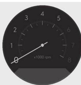
The tachometer indicates the approximate number of engine revolutions per minute (RPM).
