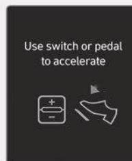
In traffic, your vehicle will stop if the vehicle ahead of you stops. Also, if the vehicle ahead of you starts moving, your vehicle will start as well. In addition, after the vehicle has stopped and a certain time have passed, the "**Use switch or pedal to accelerate**" message will appear on the instrument cluster. Depress the accelerator pedal or operate the + switch, - switch or (II) switch to start driving.
