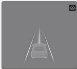
If the vehicle ahead and/or both lane markings are detected and your vehicle speed is below 120 mph (200 km/h), the green (⊖) indicator light appears on the instrument cluster, and Lane Following Assist helps center the vehicle in the lane by assisting the steering wheel.
