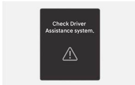
When Safe Exit Warning is not working properly, the "**Check Driver Assistance system.**" warning message will appear on the instrument cluster for several seconds, and the master warning light (Δ) will appear on the instrument cluster. If this occurs, have your vehicle inspected by an authorized HYUNDAI dealer.
