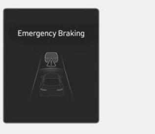
To warn the driver that emergency braking will be assisted, the "**Emergency Braking**" warning message appears and the (⚠) warning light blinks on the instrument cluster with a warning sound and the steering wheel vibrates.
