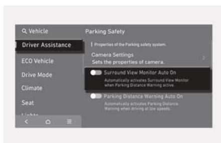
With the engine on, select **Driver Assistance > Parking Safety > Surround View Monitor Auto On** from the Settings menu in the infotainment system to use the function.
