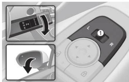
When the gear is shifted to the R (Reverse) position, the side view mirrors rotate downwards to aid with driving in reverse.
