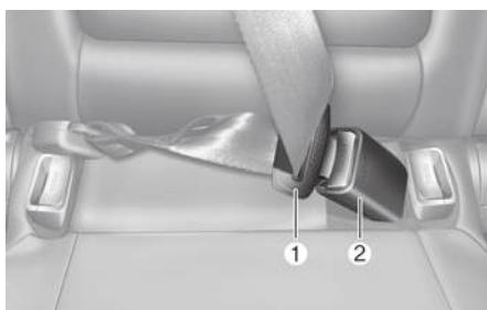
Insert the tongue plate (1) into the buckle (2) until an audible "click" is heard, indicating the latch is locked. Pull the shoulder portion of the belt to snug the belt across your hips and remove slack. Make sure the seat belt is not twisted. When using the rear center seat belt, use the buckle with the "CENTER" mark.
