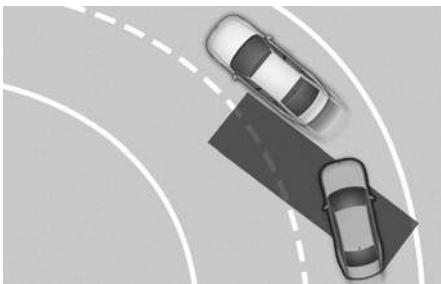
Blind-Spot Collision-Avoidance Assist may not operate properly when driving on a curved road. The function may recognize a vehicle in the same lane.
