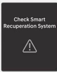
If the rear radar is covered by any foreign material, such as snow, rain, or dirt, the detecting performance may decrease and disable the smart recuperation system.
