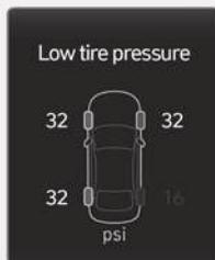
When the Tire Pressure Monitoring System warning indicator (⚠) is illuminated and a warning message appears on the cluster display, one or more of your tires is significantly under-inflated. The Low Tire Pressure Position Telltale will indicate which tire is significantly under inflated by illuminating the corresponding parking light.
