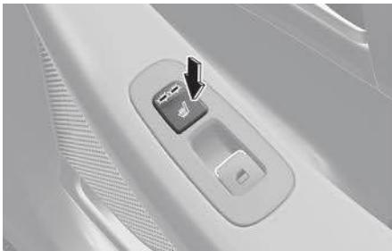
While the engine is running, press the seat warmer switch to warm the rear seats.
