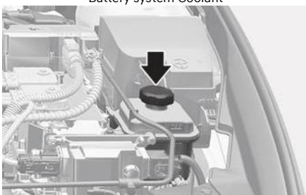
Check the condition and connections of all cooling system hoses and heater hoses. Replace any swollen or deteriorated hoses.
