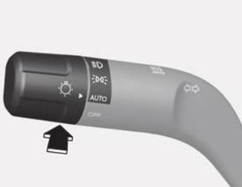
To turn on the high beam headlight, push the lever away from you. The lever returns to its original position.
