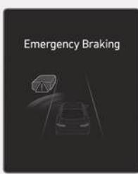
To warn the driver that emergency braking will be assisted, the "**Emergency Braking**" warning message appears and the (⚠) warning light blinks on the instrument cluster with a warning sound and the steering wheel vibrates.
