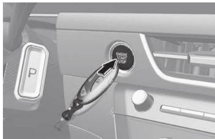
To start the engine, press the Engine Start/Stop button directly with the smart key. If you have a problem with the smart key, contact an authorized HYUNDAI dealer.
