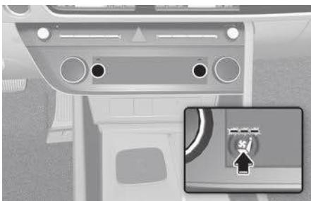
2. When you press the button, it is in the high, and you can move it in the order of medium, low, and off by pressing the button.
