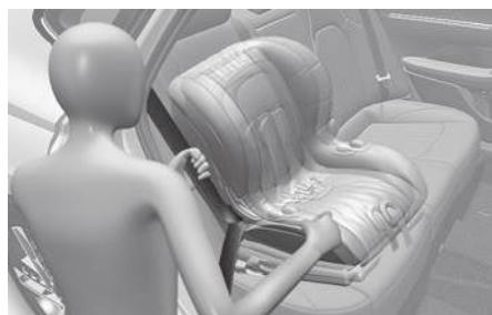
6. Push and pull on the Child Restraint System to confirm that the seat belt is holding it firmly in place. If it is not, release the seat belt and repeat steps 2 through 6.
