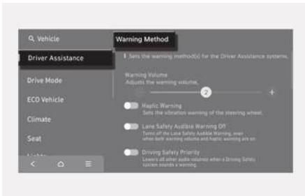
The Warning Method can be set with the engine on.
