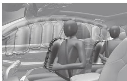
Side airbags are located in each front seat and outboard rear seats.
