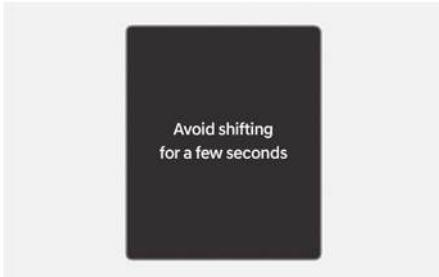
Repeated sudden acceleration and quick start may temporarily overheat the transmission. Wait until the system to cool before operating the rotary gear shift dial.
