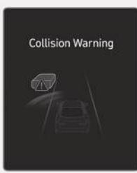
To warn the driver of a collision, the "**Collision Warning**" warning message appears and the (⚠) warning light blinks on the instrument cluster with a warning sound and the steering wheel vibrates.
