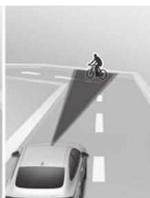
Forward Collision-Avoidance Assist may not detect a vehicle, a powered two-wheeler, a pedestrian, or a cyclist in front of you when driving on curved roads adversely affecting the performance of the sensors. This may result in no warning, braking assist when necessary.
