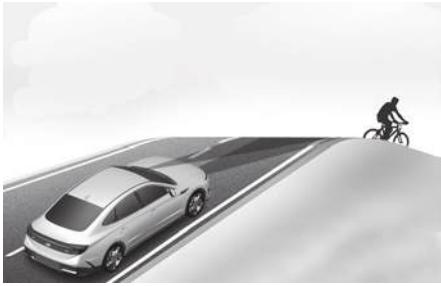
Forward Collision-Avoidance Assist may not detect a vehicle, a powered two-wheeler, a pedestrian, or a cyclist in front of you while driving uphill or downhill, adversely affecting the performance of the sensors.
