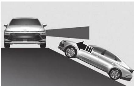
Rear Cross-Traffic Collision-Avoidance Assist may be limited when the vehicle is on an uphill or downhill slope, or near it, and may not detect the vehicle approaching from the left or right. If this occurs, the function may not warn the driver or control the brakes when necessary.
