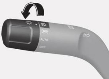
The headlight, parking light, license plate light and instrument panel lamp are turned ON.
