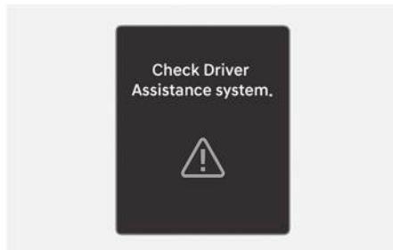
When Lane Following Assist is not working properly, the **Check Driver Assistance system** warning message will appear on the instrument cluster for several seconds, and the master (Δ) warning light appears on the instrument cluster. If this occurs, have your vehicle inspected by an authorized HYUNDAI dealer.
