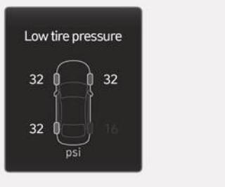
This warning message appears if the tire pressure is low. The corresponding tire on the vehicle is illuminated.
