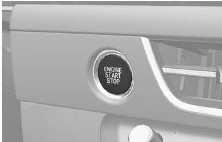
Whenever the front door is opened, the Engine Start/Stop button illuminates and goes off for a few seconds after the door is closed.
