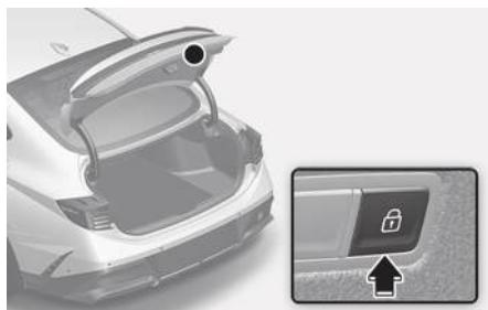
Press the power trunk lock button while carrying the Smart key. The power trunk closes and locks automatically.
