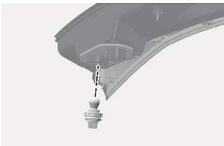
5. Remove the bulb from the socket by pressing it in and rotating it counterclockwise until the tabs on the bulb align with the slots in the socket. Pull the bulb out of the socket.
