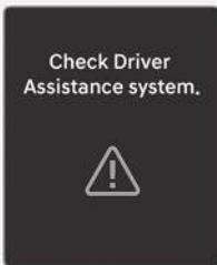
When Smart Cruise Control is not working properly, the "**Check Driver Assistance system.**" warning message and the master (⚠) warning light will appear on the instrument cluster. Have your vehicle inspected by an authorized HYUNDAI dealer.
