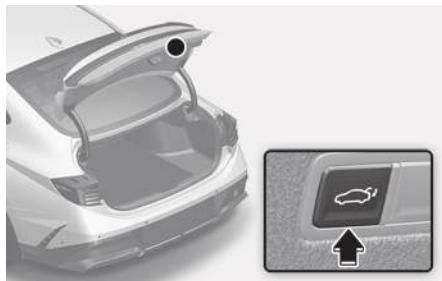
Press the power trunk close button. The trunk will close automatically.
