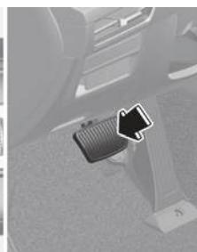
Press the (II) switch or depress the brake pedal to temporarily cancel Smart Cruise Control.
