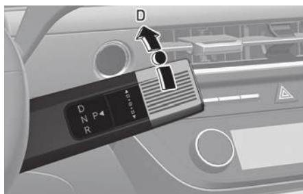
This is the normal forward driving position. The transmission automatically shift through an six gear sequence, providing the better fuel economy and power.
