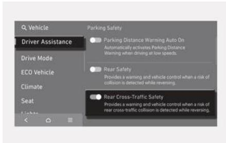
With the engine on, select **Setup > Vehicle > Driver Assistance > Parking Safety > Rear Cross-Traffic Safety** from the settings menu in the infotainment system to turn on Rear Cross-Traffic Collision-Avoidance Assist and deselect to turn off the function.
