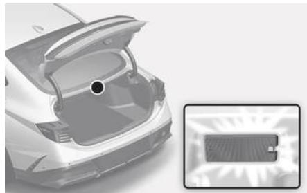
The Luggage compartment lamp turns on when the trunk is opened and off when the trunk is closed.
