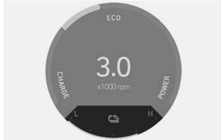
This gauge indicates the remaining hybrid battery power. If the SOC is near the L (Low) level, the vehicle automatically operates the engine to charge the battery.
