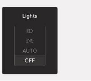
This indicator displays which exterior light is selected using the lighting control.
