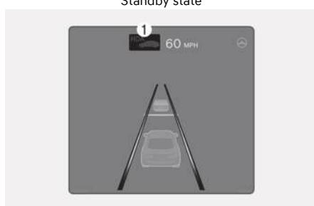
1. Highway Driving Assist indicator, whether there is a vehicle ahead and the selected distance level are displayed.
