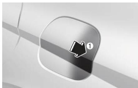
3. Pull the fuel filler door (1) outward to access the fuel tank cap.
