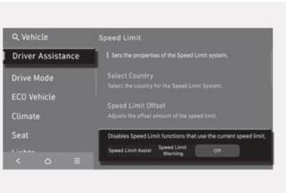
With the engine on, select or deselect **Setup > Vehicle > Driver Assistance > Speed Limit** from the Settings menu to set whether to use each function.
