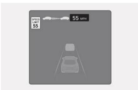
Manual Speed Limit Assist or Smart Cruise Control assists the vehicle to adjust its speed according to the speed limit. When the cruising speed is set as same as the speed limit, the vehicle automatically adjusts its speed if the speed limit changes. The function operates on the road which has a speed limit of 45 mph (70 km/h) or higher. When the function is active, the cruising speed on the instrument cluster appears in green.
