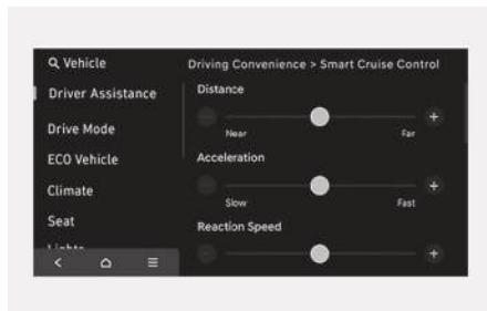
With the engine on, select **Setup > Vehicle > Driver Assistance > Driving Convenience > Smart Cruise Control** from the settings menu in the infotainment system to change Distance, Acceleration, Reaction Speed manually.
