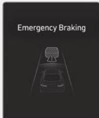
To warn the driver that emergency braking will be assisted, the "**Emergency Braking**" warning message appears and the (⚠) warning light blinks on the instrument cluster with a warning sound and the steering wheel vibrates.
