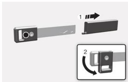
Turn the knob (2) of the mechanical key after removing the key protector (1).
