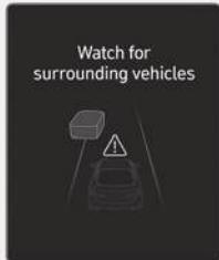
In the following situation, the "**Watch for surrounding vehicles**" warning message will appear on the instrument cluster, and an audible warning will sound to warn the driver of road conditions ahead.
