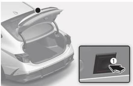
2. Start the vehicle within 30 seconds after pressing the **12V BATT RESET** button.
