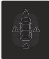
When the Parking Distance Warning is operating, if the function is not working normally or the ultrasonic sensor is blocked, the master warning light (⚠) appears in the direction of the corresponding sensor. You can check the warning in the Utility view on the cluster.
