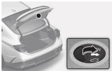
Your vehicle is equipped with an emergency trunk safety release lever located inside the trunk. When someone is inadvertently locked in the trunk, the trunk can be opened by moving the lever in the direction of the arrow and pushing the trunk lid to open.
