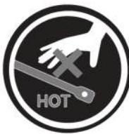
Do not touch metal parts (including strut bars) while the engine is operating or hot to prevent serious injury. Turn off the engine and wait until the metal parts cool down before working on the vehicle.
