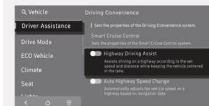
With the engine on, select or deselect **Setup > Vehicle > Driver Assistance > Driving Convenience** from the Settings menu to set whether to use each function.
