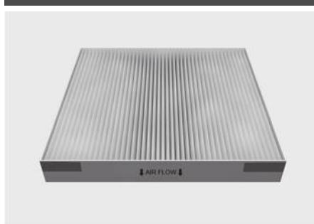
Install a new cabin air filter in the correct direction with the arrow symbol (↓) facing downwards, to prevent noise and efficiency loss.
