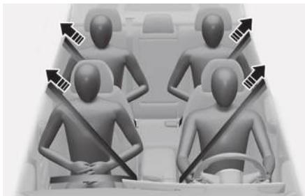
Your vehicle is equipped with driver's, front passenger's and rear passengers pretensioner seat belts (retractor pretensioner). The pretensioner makes sure the seat belts fit tightly against your body in certain frontal or side collision(s). The pretensioner seat belts may be activated in some crashes where the frontal or side collision(s) is severe enough, together with the airbags.
