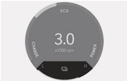
The SOC gauge indicates the remaining hybrid battery power.
