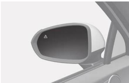
Your vehicle is equipped with both left-hand and right-hand side view mirrors. The mirrors can be adjusted with the mirror adjustment control switch. Adjust the side view mirrors to your desired position before driving. The side view mirrors can be folded to help prevent damage when going through an automatic car wash or when passing through a narrow street.
