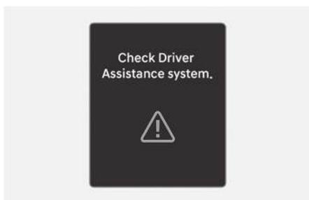
When Rear Cross-Traffic Collision-Avoidance Assist is not working properly, the "**Check Driver Assistance system.**" warning message appears on the instrument cluster for several seconds, and the master (Δ) warning light illuminates on the instrument cluster. If this occurs, have your vehicle inspected by an authorized HYUNDAI dealer.
