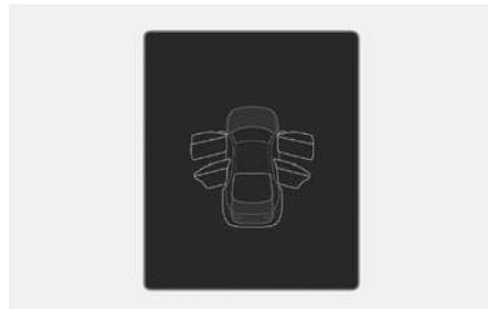
This warning appears if any door or hood or trunk is left open. The warning indicates which door is open on the cluster display.
