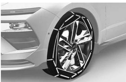
Since the sidewalls of radial tires are thinner than other types of tires, they may be damaged by mounting some types of tire chains on them. Therefore, the use of snow tires is recommended instead of tire chains. If tire chains must be used, install the tire chains after reviewing the instructions provided with the tire chains. Damage to your vehicle caused by improper tire chain use is not covered by your vehicle manufacturer's warranty.
