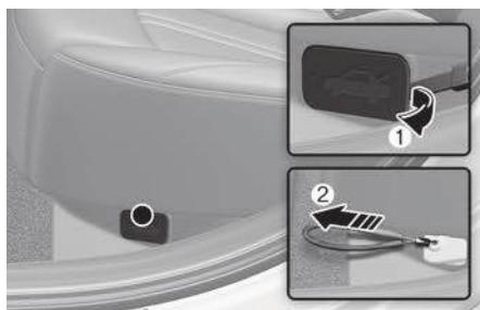
Follow the below procedure to open the power trunk manually when the battery is discharged or when there is a problem with the vehicle:
