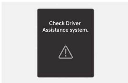
When Intelligent Speed Limit Assist is not working properly, the "**Check Driver Assistance system.**" warning message will appear on the instrument cluster for several seconds, and the master (△) warning light and speed limit (⊖) warning light will appear on the instrument cluster. If this occurs, have your vehicle inspected by an authorized HYUNDAI dealer.
