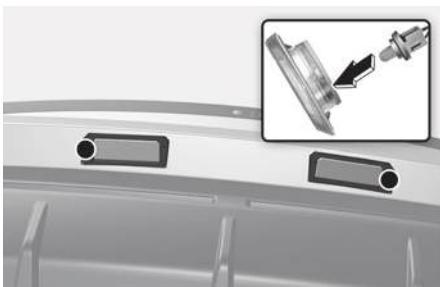
1. Using a flat-blade screwdriver, gently pry the lens cover from the lamp housing.
