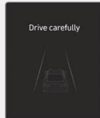
When the vehicle is stopped due to emergency braking, the "**Drive carefully**" warning message will appear on the instrument cluster.
