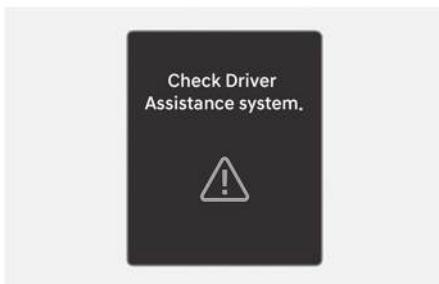
When High Beam Assist is not working properly, the "**Check Driver Assistance system**" warning message may appear, and the  $\Delta$  warning light may illuminate on the instrument cluster. Have the system inspected by an authorized HYUNDAI dealer.
