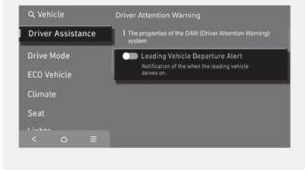
With the engine on, select **Setup** > **Vehicle** > **Driver Assistance** > **Driver Attention Warning** and then enable **Leading Vehicle Departure Alert** in the infotainment system to use the function. If **Leading Vehicle Departure Alert** is enabled, the function informs the driver when a detected vehicle in front departs from a stop.
