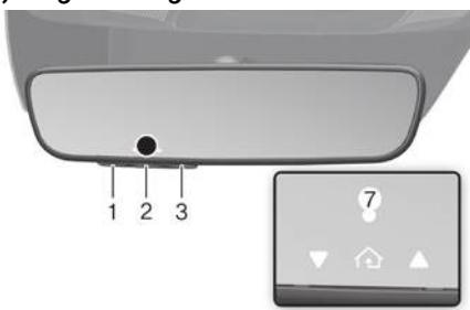
1. Press and release the HomeLink button (1), (2) or (3), you would like to program. The HomeLink indicator light (7) will flash orange slowly (if not, perform the steps of "Erasing HomeLink Buttons" section, and start over).
