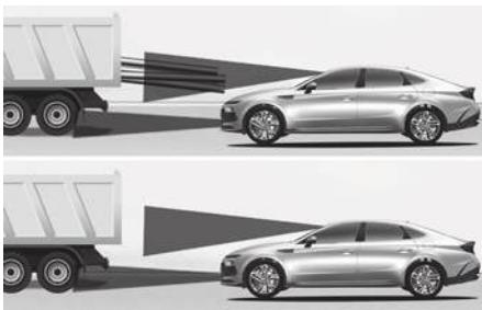
If the vehicle in front of you has cargo that extends rearward from the cab, or when the vehicle in front of you has higher ground clearance, additional special attention is required. Forward
