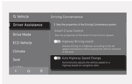
With the engine on, select **Setup > Vehicle > Driver Assistance > Driving Convenience > Auto Highway Speed Change** from the Settings menu to turn on Navigation-based Smart Cruise Control and deselect to turn off the function.
