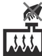
Never remove the radiator cap or the drain plug while the engine and radiator are hot. Hot coolant and steam may blow out under pressure, causing serious injury.
