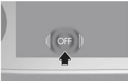
Press the **OFF** button to turn the climate control system off. You can still operate the mode and air intake buttons as long as the Engine Start/Stop button is in the ON position.
