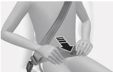
The seat belt automatically adjusts to the proper length after the lap belt portion is adjusted manually so that it fits snugly around your hips. If you lean forward in a slow, easy motion, the belt extends and moves with you.
