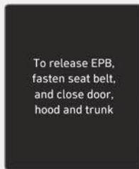
If the driver's seat belt is unfastened, or the hood, trunk, doors are open, and you try to drive with EPB applied, a warning sounds and a message appears.
