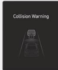
While Smart Cruise Control is operating, when the collision risk with the vehicle ahead is high, the "**Collision Warning**" warning message will appear on the instrument cluster with a warning sound and the steering wheel will vibrate to warn the driver. Always have your eyes on the road while driving, and if necessary, depress the brake pedal to reduce your driving speed in order to maintain a safe distance.
