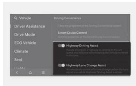
With the engine on, select or deselect **Setup > Vehicle > Driver Assistance > Driving Convenience > Highway Driving Assistance** from the infotainment system to set whether to use each function.
