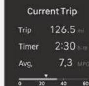
The trip computer mode displays information related to vehicle driving parameters including fuel economy, trip meter information, and vehicle speed.
