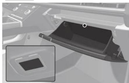
The glove box lamp turns on when the glove box is opened.
