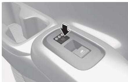
While the engine is running, press the seat warmer button to warm the rear seat.
