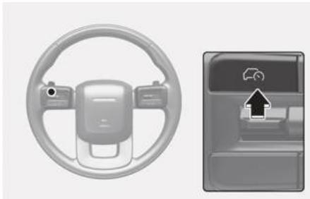
To turn Smart Cruise Control off, press the Driving Assist (
