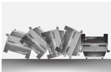
Front airbags may not inflate in rollover crash because front airbag deployment would not provide additional occupant protection.
