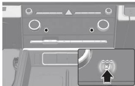
While the engine is running, touch the icon to cool the driver's seat or front passenger's seat.
