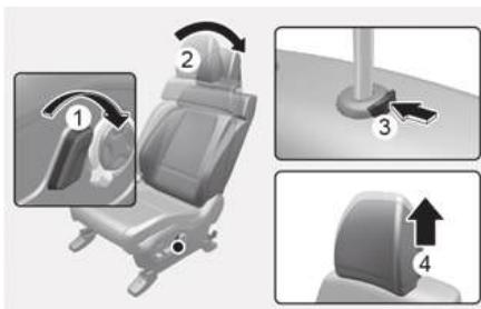
To remove the head restraint:
