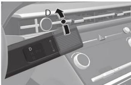
This is the normal driving position. The transmission automatically shifts through a 6 gear sequence, providing the best fuel economy and power.
