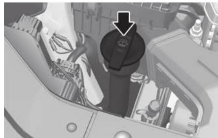
Check the fluid level in the washer fluid reservoir and add fluid if necessary. Plain water can be used during summer months if washer fluid is not available. However, use washer fluid with antifreeze in cold climates to prevent freezing.
