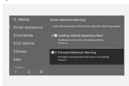
If "**Forward Attention Warning**" is enabled, the function warns the driver when the driver's gaze is not focused on the road.
