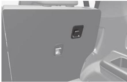
Hooks are located on the back of the 1st and 2nd row seatbacks.
