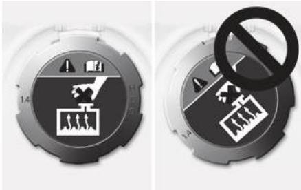
2. Make sure that the tiny protrusions inside the coolant cap are securely interlocked.
