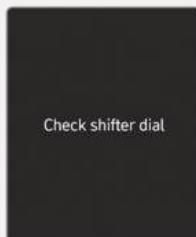
This message appears when there is a malfunction with the rotary gear shift dial. Have your vehicle inspected by an authorized HYUNDAI dealer.
