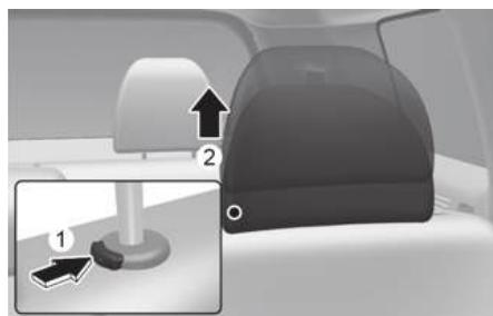
To remove the head restraint:
