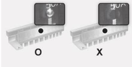
A vehicle's electrical system is protected from electrical overload damage by fuses.
