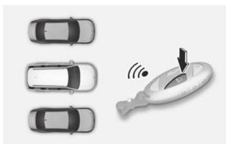
2. Press and hold the Remote Start button (hold) within 4 seconds until the vehicle starts.
