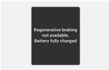
Regenerative braking is temporarily limited to protect the battery because the high voltage battery is fully charged.
