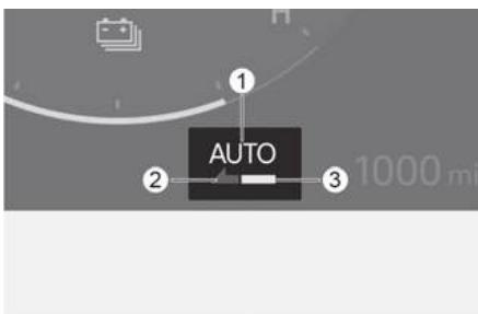
When the smart regeneration system is ON, the regenerative braking level appears as "AUTO" on the instrument cluster. The "AUTO" appears in grey in the ready state. The system automatically controls the regenerative braking level (2) according to the smart regeneration system operating conditions. If the front radar detects a vehicle in front, the indicator light (3) appears in green.
