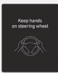
If the driver takes their hands off the steering wheel for several seconds, the "**Keep hands on steering wheel**" warning message appears on the instrument cluster, and an audible warning sounds in stages.
