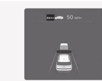
When Based on driving style is operating, the vehicle distance level and target distance will be displayed white based on the driving style.
