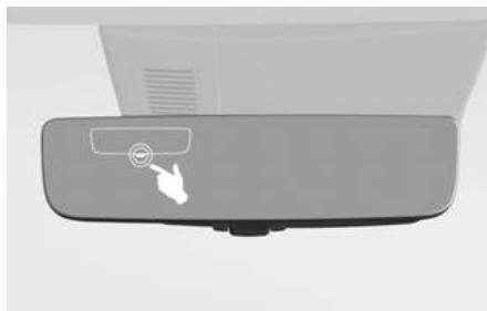
If the symbol shown in the illustration is displayed when using the Digital Center Mirror in digital mirror mode, the system may be malfunctioning. The symbol will disappear in a few seconds.
