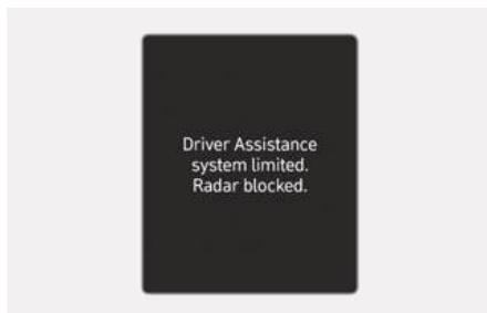
When the rear bumper around the rear corner radar or sensor is covered with foreign material, such as snow or rain, or installing a trailer or carrier, it can reduce the detecting performance and temporarily limit or disable Blind-Spot Collision-Avoidance Assist.
