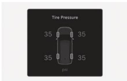
The tire pressure of each tire appears. For more information, refer to the "Tire Pressure Monitoring System (TPMS)" section in chapter 8.
