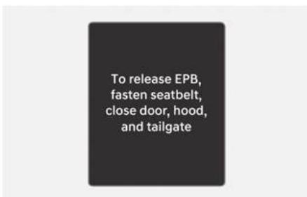
If the driver's seat belt is unfastened, or the hood, liftgate, doors are open, and you try to drive with EPB applied, a warning sounds and a message appears.
