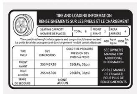
The label located on the driver's door jamb shows the original tire size, cold tire pressures recommended for your vehicle, the number of people that can be in your vehicle and vehicle capacity weight.
