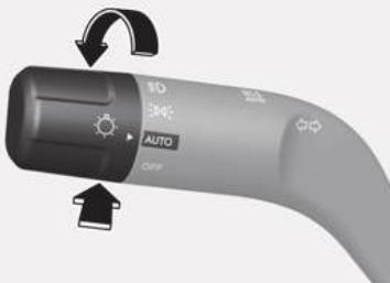
High Beam Assist automatically adjusts the headlights between high beam and low beam depending on the light detected from oncoming vehicles or vehicles in front using the front view camera.
