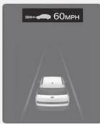
The current operation condition of Manual Speed Limit Assist, Smart Cruise Control, Lane Following Assist, etc. appears.
