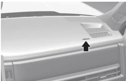
The SRS consists of advanced airbags located in the center of the steering wheel and the passenger's side front panel pad above the glove box.
