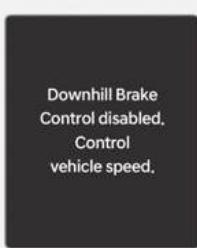
If Downhill Brake Control is not working properly, this warning message appears on the cluster display and you may hear a warning sound. If this occurs, control the vehicle speed by depressing the brake pedal.
