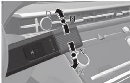
The wheels and transmission are not engaged.
