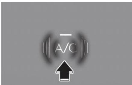
Press the **A/C** button to manually turn on the air conditioning system (indicator light ON) and off.
