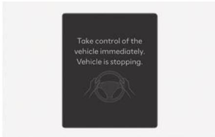
To warn you that Emergency Stop is operating the **"Take control of the vehicle immediately. Vehicle is stopping."** warning message appears on the instrument cluster, an audible warning sounds, and the steering wheel vibrates.
