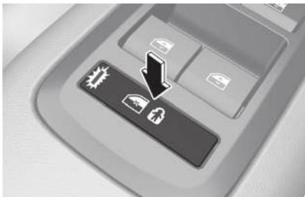
When the electronic child safety lock (🔒) button is in the LOCK position and an approaching vehicle from the rear area is detected, the electronic child safety lock button will not unlock even if the driver presses the button to prevent the rear doors from opening.
