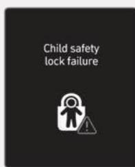
When electronic child safety lock does not work even though the button is pressed, the message will be displayed and an alarm will sound. If this occurs, have your vehicle inspected by an authorized HYUNDAI dealer.
