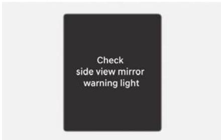
When the side view mirror warning light is not working properly, the "**Check side view mirror warning light**" warning message will appear on the instrument cluster for several seconds, and the master (Δ) warning light will illuminate on the instrument cluster. If this occurs, have your vehicle inspected by an authorized HYUNDAI dealer.
