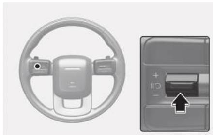
Press the **II** switch to temporarily pause the set speed limit. The set speed limit will turn off but the Speed Limit (**LIMIT**) indicator will stay on.
