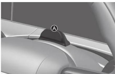
The in-cabin camera is mounted to the steering wheel.
