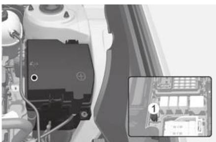
6. Check the removed fuse and replace it if it is blown. Spare fuses are provided in the instrument panel fuse panels (or in the engine compartment fuse panel).
