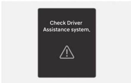
When Blind-Spot Collision-Avoidance Assist is not working properly, the "**Check Driver Assistance system.**" warning message will appear on the instrument cluster for several seconds, and the master (Δ) warning light will appear on the instrument cluster. If this occurs, have your vehicle inspected by an authorized HYUNDAI dealer.
