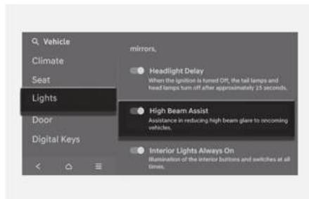
With the Engine Start/Stop button ON, go to the Settings menu to turn on High Beam Assist and deselect to turn off the function in the infotainment system.
