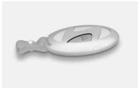
2. Press the Remote Start button (5) for more than 2 seconds on the smart key within 4 seconds from when you have pressed the door lock button. The hazard warning flasher blink and the engine starts.
