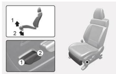
Push the control switch forward (1) to raise the leg support.
