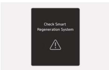
If the rear radar is covered by any foreign material, such as snow, rain, or dirt, the detecting performance may decrease and disable the smart regeneration system.
