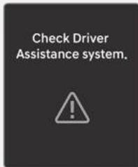
When High Beam Assist is not working properly, the "**Check Driver Assistance system**" warning message may appear, and the  $\triangle$  warning light may illuminate on the instrument cluster. Contact an authorized HYUNDAI dealer.
