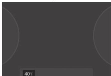
The outside ambient temperature appears in the lower portion of the cluster display. The temperature reads in Fahrenheit or Celsius depending on the units selected from the instrument cluster or infotainment system.
