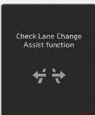
When Highway Driving Assist is not working properly, the "**Check Driver Assistance system.**" or "**Check Lane Change Assist function**" warning message and Master (⚠) warning light appears on the instrument cluster. If this occurs, have your vehicle inspected by an authorized HYUNDAI dealer.
