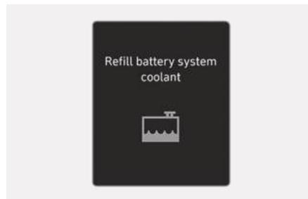
This message appears when the battery system coolant is nearly empty.
