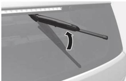
3. Press the wiper blade slot (1). Then remove the wiper blade (2).
