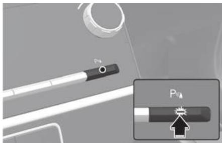
Press the Parking Safety (P $\Delta$ ) button to turn on Forward/Reverse Parking Distance Warning. Press the button again to turn off the function.
