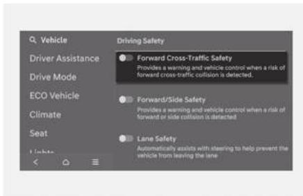
With the engine on, select **Setup > Vehicle > Driver Assistance > Forward Cross-Traffic Safety** in the infotainment system to turn on Junction Crossing function and deselect to turn off the function.
