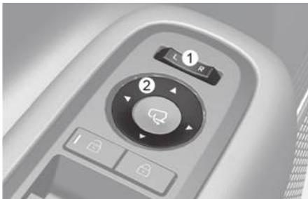
1. Press the switch (1) either to the L (left side) or R (right side) to select the side view mirror you want to adjust.
