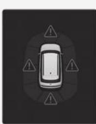
When the Parking Distance Warning is operating, if the function is not working normally or the ultrasonic sensor is blocked, the master warning light (▲) appears in the direction of the corresponding sensor. You can check the warning in the Utility view on the cluster.
