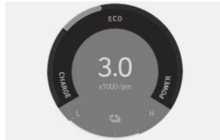
The hybrid system gauge indicates whether the current driving condition is fuel efficient or not.
