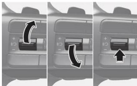
To resume Manual Speed Limit Assist after the function was paused, operate the **+**, **-**, **II** switch.
