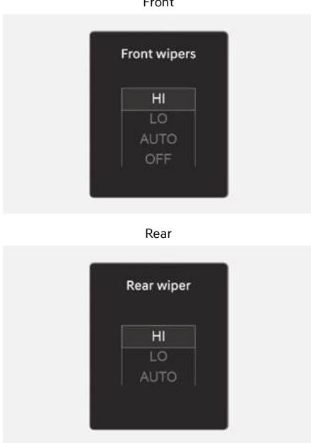
This indicator displays which wiper speed is selected using the wiper control.
