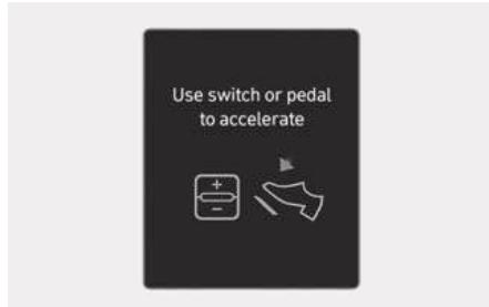
When Highway Driving Assist is operating, your vehicle will stop if the vehicle ahead of you stops. Also, if the vehicle ahead of you starts moving within 30 seconds after the stop, your vehicle will start as well. In addition, after the vehicle has stopped and 30 seconds have passed, the "**Use switch or pedal to accelerate**" message will appear on the instrument cluster. Depress the accelerator pedal or operate the + switch, - switch or II/C switch to start driving.
