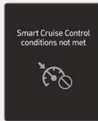
If the Driving Assist button, + switch, - switch or II $\odot$  switch is operated when Smart Cruise Control operating conditions are not satisfied, the "**Smart Cruise Ctrl. conditions not met**" will appear on the instrument cluster, and an audible warning will sound.
