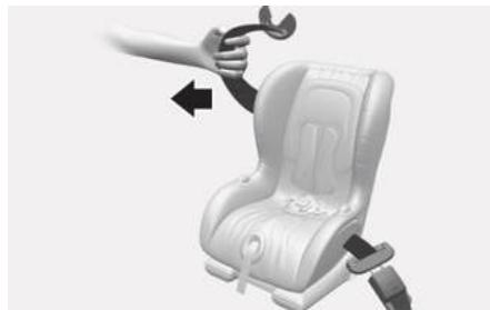
4. Slowly allow the shoulder portion of the seat belt to retract and listen for an audible "clicking" or "ratcheting" sound. This indicates that the retractor is in the Automatic Locking mode. If no distinct sound is heard, repeat Step 3 and 4.
