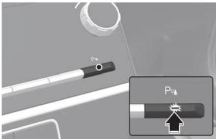
Press and hold the Parking Safety (P $\Delta$ ) button more than 2 seconds, to turn the Parking Collision-Avoidance Assist on or off.
