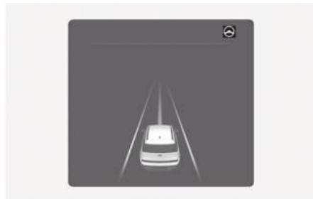
If the vehicle ahead and/or both lane markings are detected and your vehicle speed is below 110 mph (180 km/h), the green (⌚) indicator light appears on the cluster, and Lane Following Assist helps center the vehicle in the lane by assisting the steering wheel.
