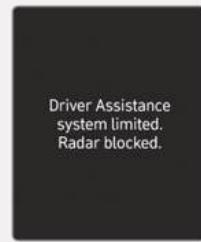
When the front radar cover or sensor is covered with snow, rain, or foreign material, it can reduce the detecting performance and temporarily limit or disable Smart Cruise Control.
