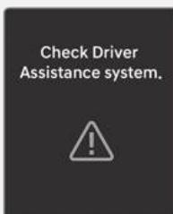
When Intelligent Speed Limit Assist is not working properly, the "**Check Driver Assistance system.**" warning message will appear on the instrument cluster for several seconds, and the master (△) warning light and (✉) warning light will illuminate on the instrument cluster. If this occurs, have your vehicle inspected by an authorized HYUNDAI dealer.
