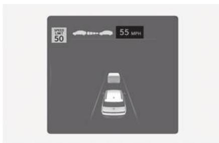
When driving at a speed higher than the displayed speed limit, the speed limit is displayed in red.
