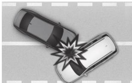
In an angled collision, the force of impact may position the occupants in a direction where the airbags would not be able to provide any additional benefit, and thus the sensors may not deploy any airbags.
