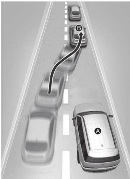
When a vehicle moves into your lane from an adjacent lane, it cannot be detected by the sensor until it is in the sensor's detection range. The smart regeneration system may not immediately detect the vehicle when your vehicle changes lanes abruptly.
