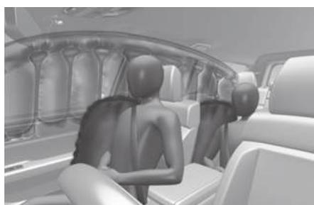
The side airbags are designed to deploy during certain side impact collisions, depending on the crash severity.
