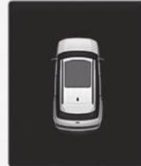
If the driver turns off the engine when the sunroof is not fully closed, the warning chime will sound for several seconds and the sunroof open warning will appear on the cluster display.
