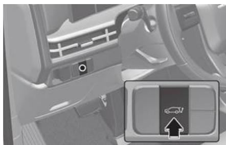
When the liftgate is closed, press the power liftgate open/close button for 1 second. The power liftgate opens with a warning sound.
