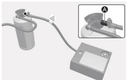
3. Unscrew the valve cap from the valve of the defective wheel and screw the filling hose (3) of the sealant bottle onto the tire valve.
