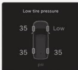
This warning message appears if the tire pressure is low. The corresponding tire on the vehicle is illuminated.
