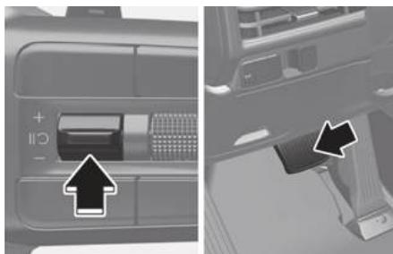
Press the **I'D** switch or depress the brake pedal to temporarily cancel Smart Cruise Control.
