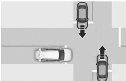
Junction Crossing function can help avoid a collision with oncoming vehicles on the left or right side when crossing an intersection by applying emergency braking.
