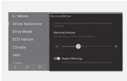
The Warning Methods can be set with the engine on. Select **Setup > Vehicle > Driver Assistance > Warning Method** from the infotainment system to change the following settings:
