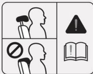
When a passenger is sitting on the 2nd row center seat, always raise the head restraint above the lowest stored position.
