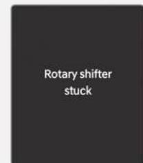
This message appears when the rotary gear shift dial does not return back to its normal position after rotating it.
