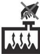
Never remove the engine coolant reservoir cap, radiator cap, or drain plug while the engine and radiator are hot. Hot coolant and steam may blow out under pressure, causing serious injury.
