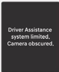
When the front windshield where the front view camera is located, or sensor is covered with foreign material, such as snow or rain, it can reduce the detecting performance and temporarily limit or disable Lane Keeping Assist.
