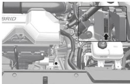
The engine number is stamped on the engine block as shown in the illustration.
