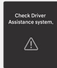
When Smart Cruise Control is not working properly, the "Check Driver Assistance system." warning message will appear, and the "⚠" warning light will illuminate on the instrument cluster. Have your vehicle inspected by an authorized HYUNDAI dealer.
