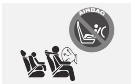
Even though your vehicle is equipped with the OCS, never install a Child Restraint System in the front passenger's seat. An inflating airbag may forcefully strike a child or child restraint resulting in serious or fatal injury.
