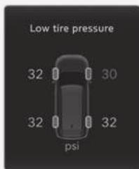
**TMPS is not a substitute for manually checking the tire pressure with a tire gauge. Changes in temperature affect tire pressure. Refer to "Check tire inflation pressure" in the Maintenance chapter for proper tire inflation and tire pressure measurement procedure.**
