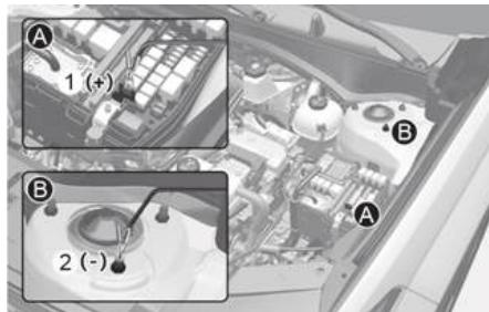
(1) RED cable : (+) jumper terminal in the engine compartment fuse panel
