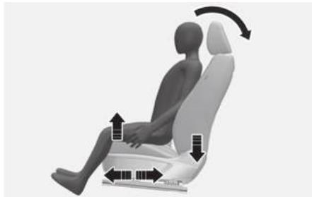
Relaxation comfort seats help distribute body pressure and concentrated weight on specific body parts that occur while sitting in the same position for a long period of time. The seat helps relieve fatigue and discomfort by providing the optimal sit position.
