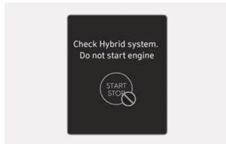
This message appears when the hybrid battery power (SOC) level is low. A warning chime will sound until the problem is solved. Refrain from driving when the warning message appears.
