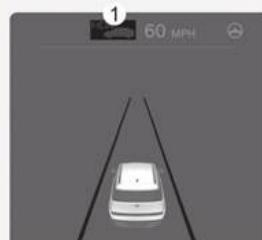
1. Highway Driving Assist indicator, whether there is a vehicle ahead and the selected distance level are displayed.
