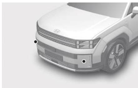
The front corner radars are mounted near the front corners of your vehicle above.
