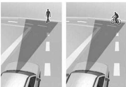
On curves, the smart regeneration system may not detect a vehicle in the same lane, and may accelerate the vehicle by lowering the regenerative braking intensity automatically. Your vehicle speed may decelerate by increasing regenerative braking intensity automatically if a vehicle is detected in an adjacent lane or when a vehicle ahead is detected suddenly. Apply the brake pedal or accelerator pedal depending on the road and driving conditions.
