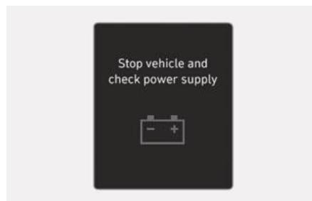
This message appears when a failure occurs in the power supply system.
