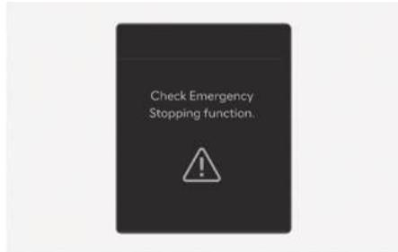
When Emergency Stop is not working properly, the "Check Emergency Stopping function." warning message appears, and the master (⚠) warning light illuminates on the instrument cluster. If this occurs, have your vehicle inspected by an authorized HYUNDAI dealer.
