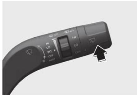
The rear wiper operates while the vehicle is in reverse with the front wiper on. You can select the function from the Settings menu in the infotainment system. Select: **Setup > Vehicle > Convenience > Auto Rear Wiper (in R)**
