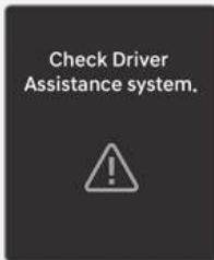
When Lane Following Assist is not working properly, the "**Check Driver Assistance system.**" warning message will appear on the instrument cluster for several seconds, and the master (⚠) warning light appears on the instrument cluster. If this occurs, have your vehicle inspected by an authorized HYUNDAI dealer.
