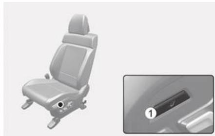
Press the front portion of the switch (1) for more than 0.5 seconds while the seat is in the relaxation comfort seat position, the seat return backs to the original position.
