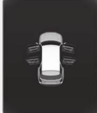
This warning is displayed if any door or hood or liftgate is left open. The warning will indicate which door is open in the display.
