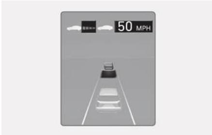
If you want to speed up temporarily without altering the set speed while Smart Cruise Control is operating, depress the accelerator pedal. While the accelerator pedal is depressed, the set speed, distance level and target distance will blink on the cluster.
