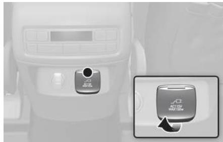
The AC inverter supplies 115 volts (150 watts) electric power to operate electric accessories or equipment.
