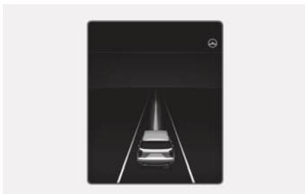
If the vehicle ahead and/or both lane markings are detected and your vehicle speed is below 120 mph (200 km/h), the green
