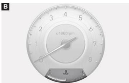
This gauge indicates the temperature of the engine coolant when the ignition switch is in the ON position.
