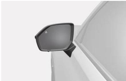
To warn the driver a vehicle is detected, the warning light on the side view mirror and head-up display (if equipped) will illuminate.
