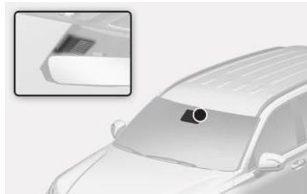
The rain sensor located on the upper end of the windshield glass senses the amount of rainfall and controls the wiping cycle for the proper interval.
