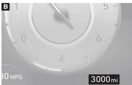
The odometer indicates the total distance that the vehicle has been driven and should be used to determine when periodic maintenance should be performed.
