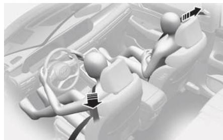
Your vehicle is equipped with driver's and front passenger's and rear passengers Pre-tensioner Seat Belts (Retractor Pre-tensioner). The purpose of the pre-tensioner is to make sure the seat belts fit tightly against the occupant's body in certain frontal or side collision(s). The pre-tensioner seat belts may be activated in crashes where the frontal or side collision(s) is severe enough, together with the air bags.
