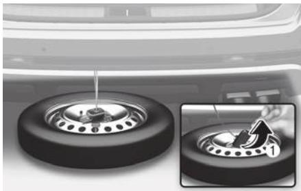
6. Draw out the retainer guide (1) through the center hole of the spare tire.
