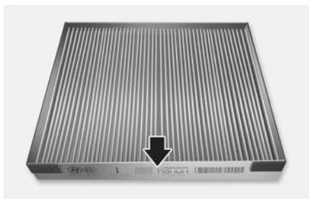
Install a new cabin air filter in the correct direction with the arrow symbol (↓) facing downwards, to prevent noise and reduce effectiveness.
