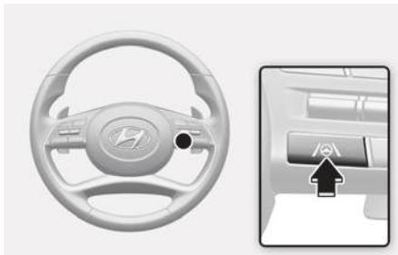
With the engine on, shortly press the Lane Driving Assist button located on the steering wheel to turn on Lane Following Assist. The grey or green
