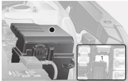
5. Pull the suspected fuse straight out. Use the removal tool (1) provided in the engine compartment fuse panel.
