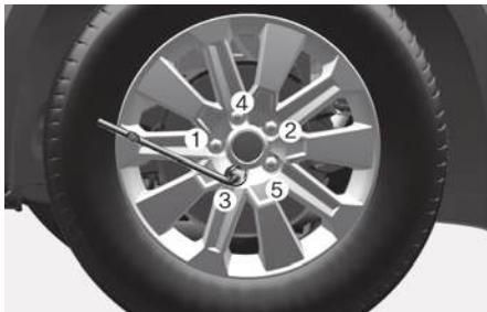
6. Loosen the wheel lug nuts counterclockwise one turn each in the order shown above, but do not remove any lug nuts until the tire has been raised off of the ground.
