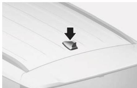
The shark fin antenna will receive AM, FM broadcast and SXM channel signals and transmit data.
