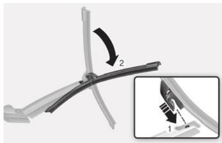
3. Install the new blade assembly by inserting the center part into the slot in the wiper arm until it clicks into place (1).
