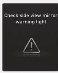
When the side view mirror warning light is not working properly, the 'Check side view mirror warning light' warning message will appear on the cluster for several seconds, and the master (▲) warning light will illuminate on the cluster. If this occurs, have the vehicle inspected by an authorized HYUNDAI dealer.
