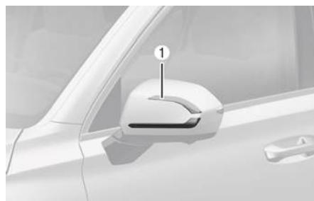
If the LED lamp (1) does not operate, have the system inspected by an authorized retailer of HYUNDAI dealer.
