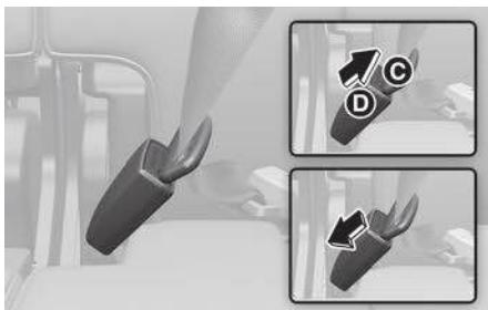
3. Pull out the tongue plate (C) from the pocket. Pull the tongue plate (C) and insert it into the buckle (D) until an audible "click" is heard, indicating the latch is locked. Make sure the belt is not twisted.
