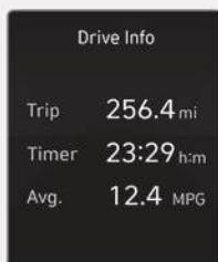
The trip computer mode displays information related to vehicle driving parameters including fuel economy, tripmeter information and vehicle speed.
