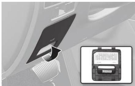
Inside the fuse/relay box cover, you can find the fuse/relay label describing fuse/relay names and ratings.
