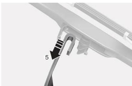
5. Remove the wiper blade from the wiper arm (5).
