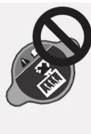
1. Check if the coolant cap label is straight in front.
