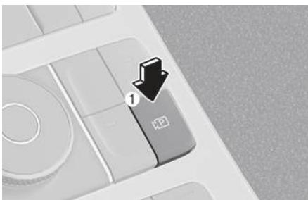
Press the Parking/View button (1) while the gear is in P (Park) to turn on Rear View Monitor.
