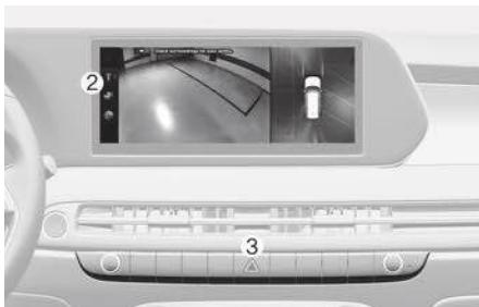
The front image is displayed on the screen when the gear is in N (Neutral) or D (Drive) to assist in parking. Using the view button (2) you may select top view, front view, side view and 3D view.
