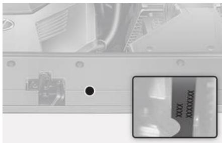
The engine number is stamped on the engine block as shown in the drawing.
