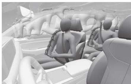
Your vehicle is equipped with a side air bag in each seat. The purpose of the air bag is to provide the vehicle's additional protection than that offered by the seat belt alone.
