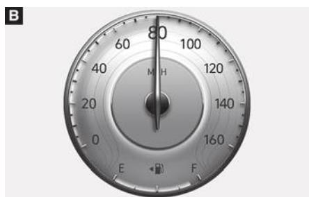
The speedometer indicates the speed of the vehicle and is calibrated in miles per hour (MPH) and/or kilometers per hour (km/h).
