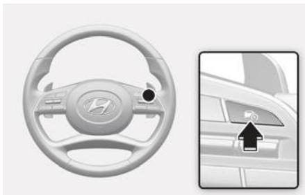
Press the Driving Assist (⌚) button to turn Smart Cruise Control off.
