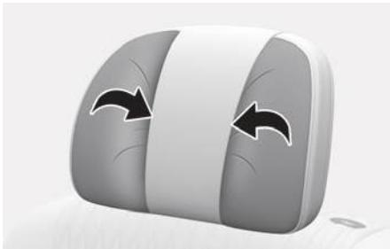
While driving, the wing-out headrest supports the passenger's head from shaking. Hold both ends of the wing-out headrest with your hands, and pull out or push in to adjust its position.
