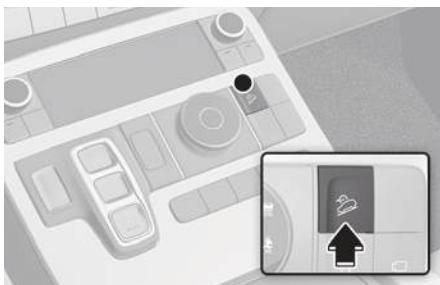
Downhill Brake Control assists the driver to descend down a steep hill without having to depress the brake pedal.
