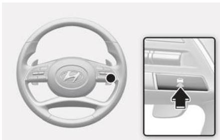
Each time the button is pressed, the headway changes as follows:
