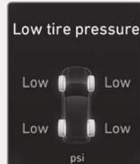
This warning message is displayed if the tire pressure is low. The corresponding tire on the vehicle will be illuminated.
