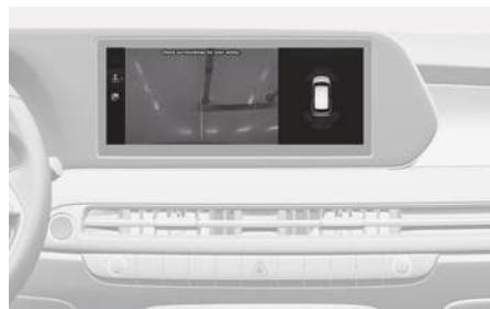
When you touch the
