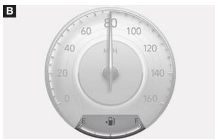
This gauge indicates the approximate amount of fuel remaining in the fuel tank.
