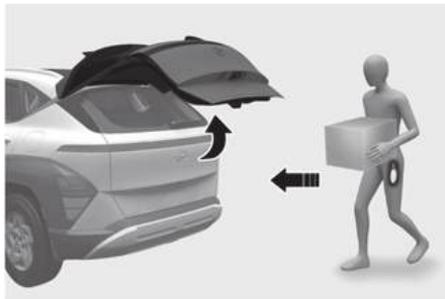
On a vehicle equipped with a smart key, the liftgate can be opened with hands-free activation using the smart liftgate system.
