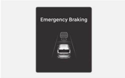
To warn the driver that emergency braking will be assisted, the "**Emergency Braking**" warning message appears and the (⚠️) warning light blinks on the instrument cluster with a warning sound and the steering wheel vibrates.
