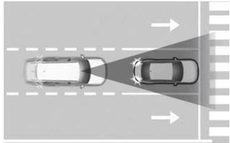
Forward Collision-Avoidance Assist helps detect a vehicle, a powered two-wheeler, a pedestrian, or a cyclist ahead on the road and may warn you of a possible collision with a warning message on the instrument cluster and a warning sound. Also, Forward Collision-Avoidance Assist may assist with braking your vehicle to help reduce collision speed or avoid a collision.
