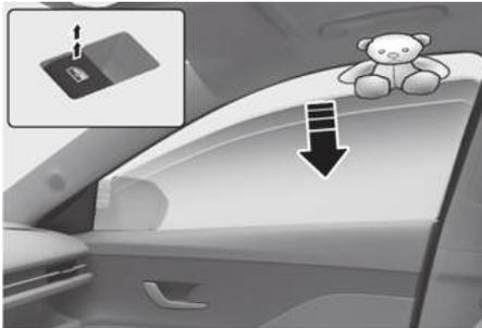
If a window senses any obstacle while it is closing automatically, it stops and lowers about 12 inches (30 cm) to allow the object to be cleared.
