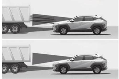
If the vehicle in front of you has cargo that extends rearward from the cab, or when the vehicle in front of you has higher ground clearance, additional special attention is required. Forward Collision-Avoidance Assist may not be able to detect the cargo extending from the vehicle. In these instances, you must maintain a safe braking distance from the rearmost object, and if necessary, steer your vehicle and depress the brake pedal to reduce your driving speed in order to maintain distance.
