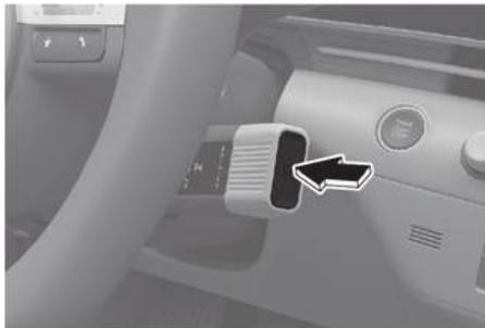
To shift the gear to P (Park), press the P button while depressing the brake pedal.
