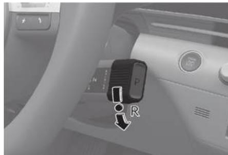
To shift the gear R (Reverse), rotate the rotary gear shift dial to R (Reverse) while depressing the brake pedal.
