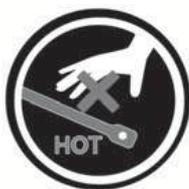
Do not touch metal parts (including strut bars) while the engine is operating or hot to prevent serious injury. Turn off the engine and wait until the metal parts cool down before working on the vehicle.
