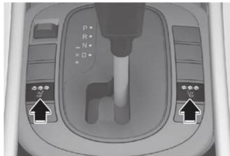
While the engine is running, press the switch to warm the driver's seat or front passenger's seat.
