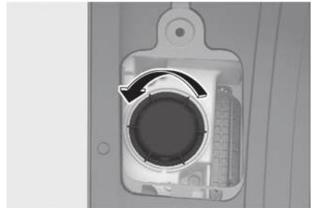
5. Remove the bulb from the socket by pressing it in and turning it counterclockwise.
