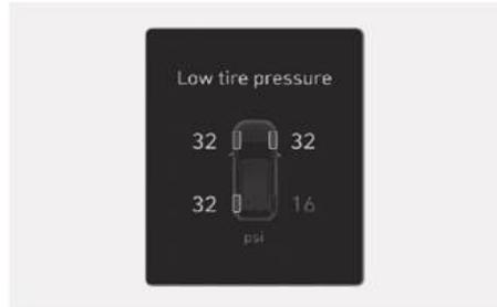
When the Tire Pressure Monitoring System warning indicator (⚠️) is illuminated and a warning message appears on the cluster display, one or more of your tires is significantly under-inflated. The Low Tire Pressure Position Telltale will indicate which tire is significantly under inflated by illuminating the corresponding parking light.
