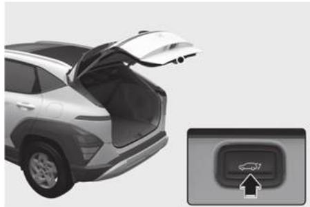
Press the power liftgate open/close button. The liftgate opens or closes automatically.
