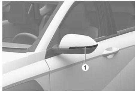
If the side repeater light (1) does not operate, have the system inspected by an authorized HYUNDAI dealer.
