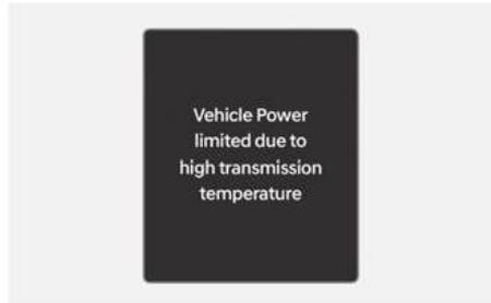
If you continue to drive with overheated transmission, the above warning message appears and self-protection mode restricts the power output of the vehicle.
