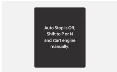
When the system is deactivated, the ISG off button indicator illuminates and a message appears on the cluster display with a warning sound if:
