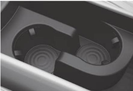
Push the button. The cup supporter protrudes from the front console. Push in the cup supporter after use.
