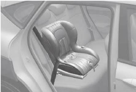
Since all passenger seat belts move freely under normal conditions and only lock under extreme or emergency conditions (emergency locking mode), you must manually pull the seat belt all the way out to shift the retractor to the "Automatic Locking" mode to secure a Child Restraint System.
