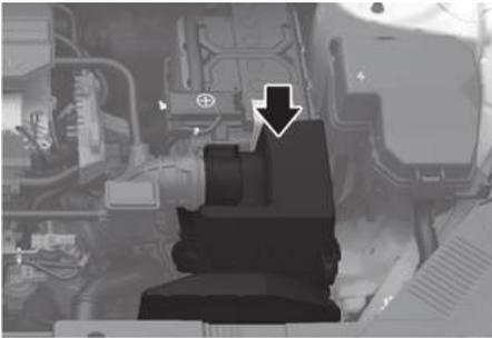
The air cleaner filter can be cleaned for inspection using compressed air.
