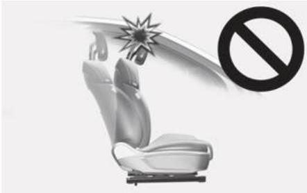
If you recline the seatback towards the front with the head restraint and seat cushion raised, the head restraint may come in contact with the sunvisor or other parts of the vehicle.
