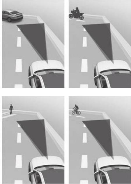
Forward Collision-Avoidance Assist may not detect a vehicle, a powered two-wheeler, a pedestrian, or a cyclist in front of you when driving on curved roads adversely affecting the performance of the sensors. This may result in no warning, braking assist when necessary.
