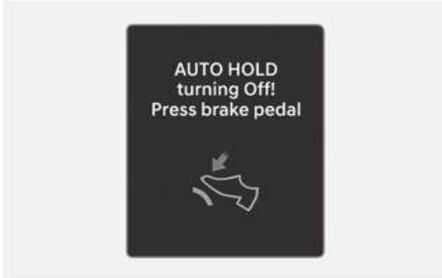
When the conversion from Auto Hold to EPB is not working properly, a warning sounds and a message appears.
