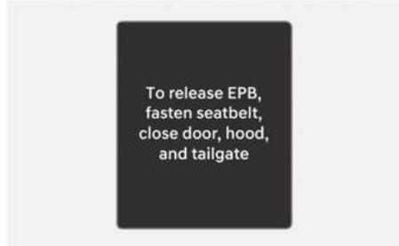
If the driver's seat belt is unfastened, or the hood, liftgate, doors are open, and you try to drive with EPB applied, a warning sounds and a message appears.
