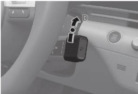
To shift the gear D (Drive), rotate the rotary gear shift dial to D (Drive) while depressing the brake pedal.
