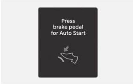
When the gear is shifted from N (Neutral) to R (Reverse), D (Drive), or Manual shift mode without the brake pedal depressed, a message appears on the cluster display. To activate auto start, depress the brake pedal.
