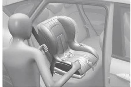
6. Push and pull on the Child Restraint System to confirm that the seat belt is holding it firmly in place. If it is not, release the seat belt and repeat steps 2 through 6.
