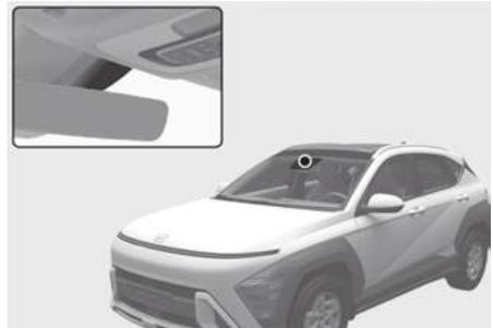
The Auto defogging reduces the possibility of fogging up the inside of the windshield by automatically sensing the moisture on inside the windshield.
