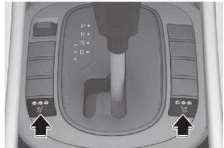
While the engine running, press the switches to cool the driver's seat or front passenger's seat.
