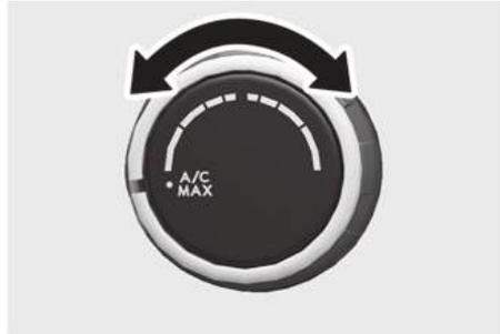
The temperature increases by turning the knob to the right. The temperature decreases by turning the knob to the left.
