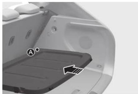
3. Insert the cargo area cover to the lower fixing part (A) on both sides.
