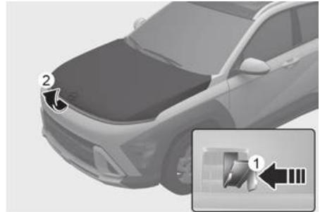
3. Go to the front of the vehicle, raise the hood slightly, push to the left the secondary hood release lever (1) inside of the hood center and lift the hood (2). After the hood has been lifted halfway, it will raise completely by itself.
