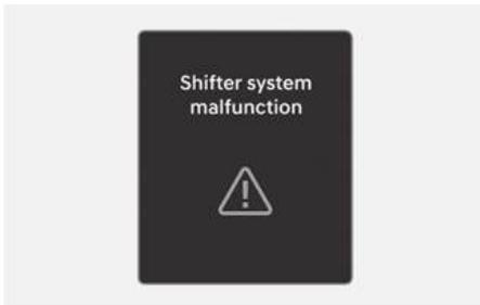
This message appears when the transmission or the shift dial does not properly operate in the P (Park) position.
