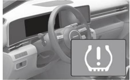
The TPMS Malfunction Indicator (
