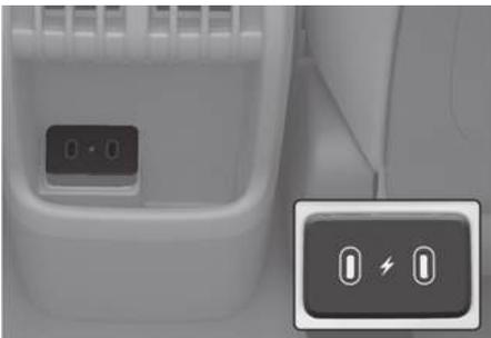
The USB charger is designed to recharge batteries of small size electronic devices using a USB cable.
