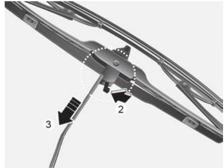
5. Install a new wiper blade assembly in the reverse order of removal.
