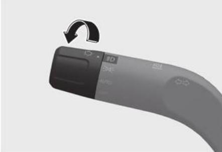
The headlight, parking light, license plate light and instrument panel lamp are turned ON.
