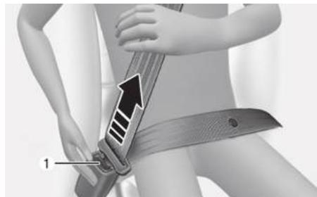
Press the release button (1) in the locking buckle.
