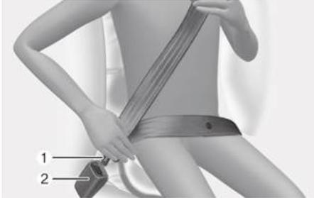
Pull it out of the retractor and insert the metal tab (1) into the buckle (2). An audible “click” sounds when the tab locks into the buckle. Make sure the seat belt is not twisted.
