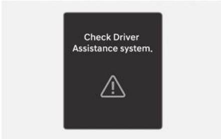
When Lane Keeping Assist is not working properly, the "**Check Driver Assistance system.**" warning message and yellow Lane Keeping Assist (LKA) warning light appears on the instrument cluster. If this occurs, have the vehicle inspected by an authorized HYUNDAI dealer.
