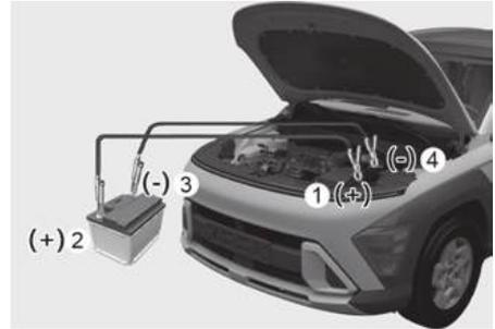
6. Connect the jumper cables in the exact sequence shown in the illustration. First connect one jumper cable to the red, positive (+) battery terminal of your vehicle (1).
