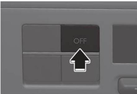
Press the OFF button to turn the climate control system off. You can still operate the mode and air intake buttons as long as the Engine Start/Stop button is in the ON position.
