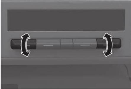
Push up the switch to increase the temperature. Push down to decrease the temperature.
