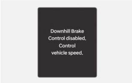
If Downhill Brake Control is not working properly, this warning message appears on the cluster display and you may hear a warning sound. If this occurs, control the vehicle speed by depressing the brake pedal.
