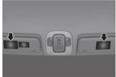
Airbag warning labels, required by the U.S. National Highway Traffic Safety Administration (NHTSA), are attached to alert the driver and passengers of potential risks of the airbag system. Be sure to read all of the information about the airbags that are installed on your vehicle in this Owner's Manual.
