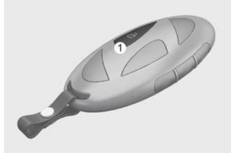
Press and hold the Door Unlock (1) button on the smart key for more than 3 seconds and the windows move down after the doors are unlocked. Window movement stops when you release the door unlock button.
