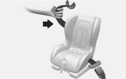
5. Remove as much slack from the belt as possible by pushing down on the Child Restraint System while feeding the shoulder belt back into the retractor.
