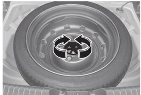
Turn the winged hold down bolt counterclockwise to remove the spare tire.
