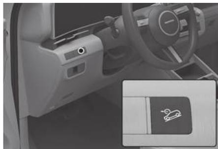
Downhill Brake Control assists when descending down a steep hill without having to depress the brake pedal.
