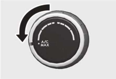
The MAX A/C mode is used to cool the inside of the vehicle faster. Air flow is directed toward the upper body and face. The air conditioning and recirculated air are both selected. Turn the fan speed mode to adjust.
