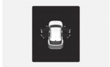
This warning appears if any door or hood or liftgate is left open. The warning indicates which door is open on the cluster display.
