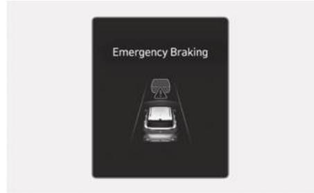
To warn the driver that emergency braking will be assisted, the "Emergency Braking" warning message appears and the (⚠️) warning light blinks on the instrument cluster with a warning sound and the steering wheel vibrates.
