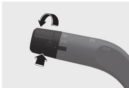
High Beam Assist automatically switches between high beam and low beam depending on the detected brightness from the lights of oncoming vehicles or vehicles in front.
