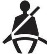
This warning light informs the driver that the seat belt is not fastened.
