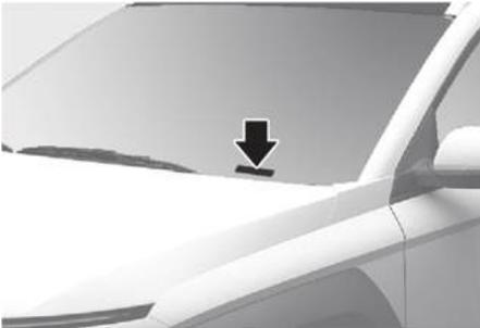
The VIN is also on a plate attached to the top of the left side dashboard. The number on the plate can easily be seen through the windshield from outside.
