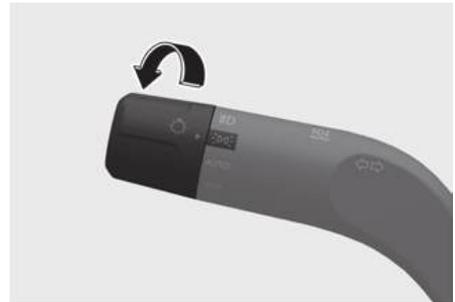
The parking light, license plate light, and instrument panel lamp are turned ON.
