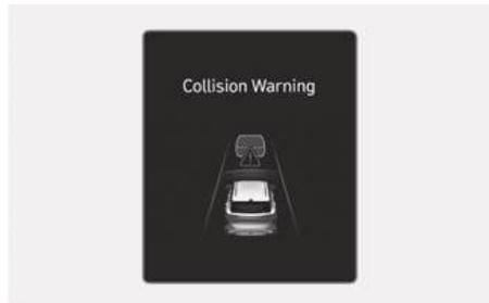
To warn the driver of a collision, the "**Collision Warning**" warning message appears and the (⚠️) warning light blinks on the instrument cluster with a warning sound and the steering wheel vibrates.
