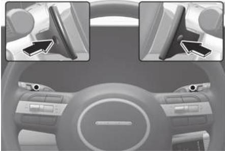
The paddle shifter is available when the gear is in the D (Drive) position.
