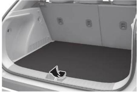
2. Remove the luggage floor and insert the luggage floor into the lower position. It may take a good push to fully seat it so it lays flat at the rear.
