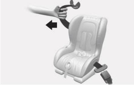
4. Slowly allow the shoulder portion of the seat belt to retract and listen for an audible "clicking" or "ratcheting" sound. This indicates that the retractor is in the "Automatic Locking" mode. If no distinct sound is heard, repeat steps 3 and 4.
