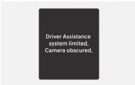
When the front windshield where the front view camera is located, or sensor is covered with foreign material, such as snow or rain, it can reduce the detecting performance and temporarily limit or disable Lane Keeping Assist.
