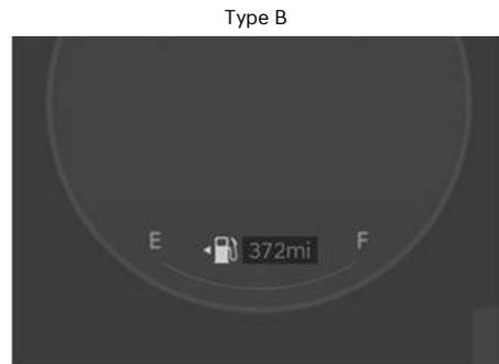
The distance to empty is the estimated distance the vehicle can be driven with the remaining fuel.
