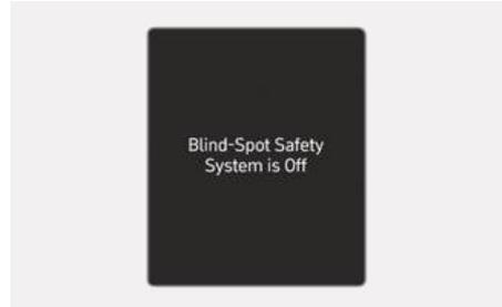
When the vehicle is restarted with Blind-Spot Collision-Avoidance Assist off, the “**Blind-Spot Safety System is Off**” message will appear on the instrument cluster.
