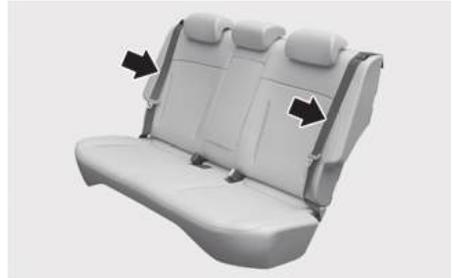
4. Pull up the seatback folding lever, then fold the seat toward the front of the vehicle.
