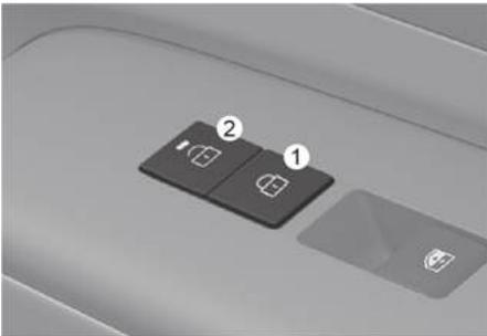
When pressing the
