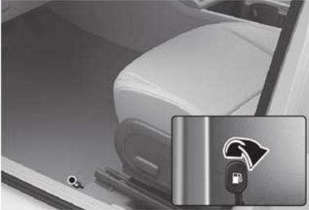
3. Pull the fuel filler door (1) outward to access the fuel tank cap.
