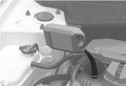
Use only the specified engine oil (Refer to the “Recommended Lubricants And Capacities” section in chapter 2).
