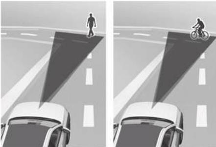
Forward Collision-Avoidance Assist may detect a vehicle, powered two-wheeler, pedestrian, or cyclist in the next lane or outside the lane when driving on a curved road.
