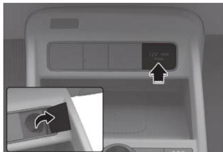
The power outlet is designed to provide power for mobile phones or other devices designed to operate with vehicle electrical systems.
