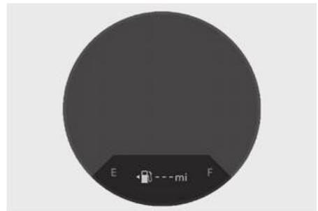
The fuel gauge indicates the approximate amount of fuel remaining in the fuel tank.
