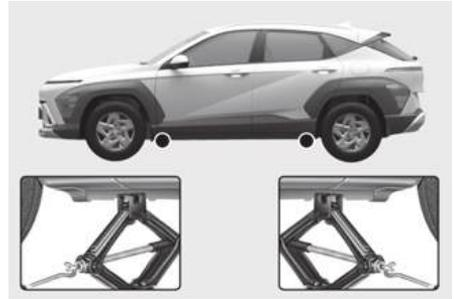
8. Insert the jack handle into the jack and turn it clockwise, raising the vehicle until the tire clears the ground. Make sure the vehicle is stable on the jack.
