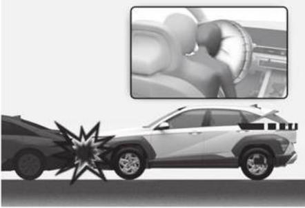
Front airbags are designed to inflate in a frontal collision depending on the severity of impact.
