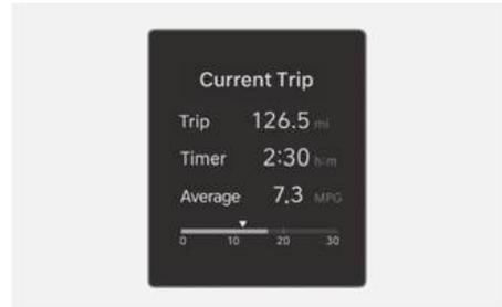
The trip computer mode displays information related to vehicle driving parameters including fuel economy, tripmeter information, and vehicle speed.
