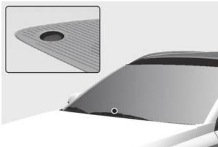
Never place anything near the sensor to ensure better control of the heating and cooling system.
