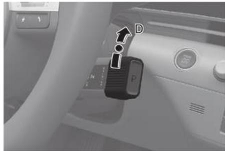
This is the normal forward driving position. The transmission automatically shifts to the optimal gear ratio, providing better fuel efficiency and a smoother ride.
