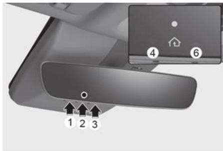
2. The indicator (4) and (6) operates as below, if your garage door opener has Two-Way Communication functionality.
