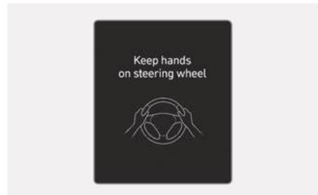
If the driver takes their hands off the steering wheel for several seconds, the "**Keep hands on steering wheel!**" warning message appears on the instrument cluster, and an audible warning sounds in stages.
