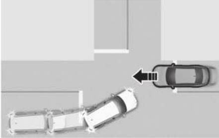
Junction Turning function can help avoid a collision with an oncoming vehicle, powered two-wheeler in an adjacent lane when turning left at a crossroad with the turn signal on by applying emergency braking.
