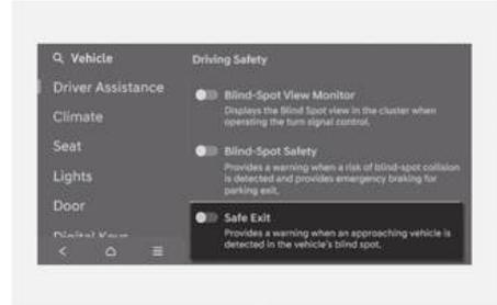
With the engine on, select **Setup** > **Vehicle** > **Driver Assistance** > **Driving Safety** > **Safe Exit** from the Settings menu to turn on Safe Exit Warning and deselect to turn off the function.
