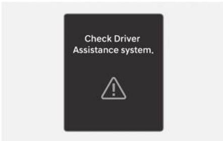
When High Beam Assist is not working properly, the "**Check Driver Assistance system**" warning message may appear, and the
