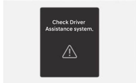
When Safe Exit Warning is not working properly, the "**Check Driver Assistance system.**" warning message will appear on the instrument cluster for several seconds, and the master warning light (
