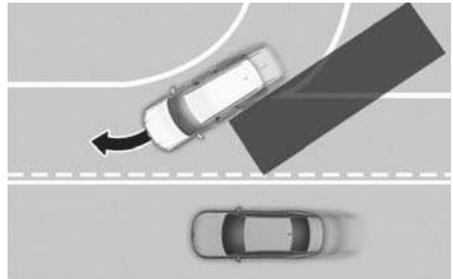
Blind-Spot Collision-Avoidance Assist may not operate properly when driving where the road merges or divides. The function may not detect the vehicle in the next lane.
