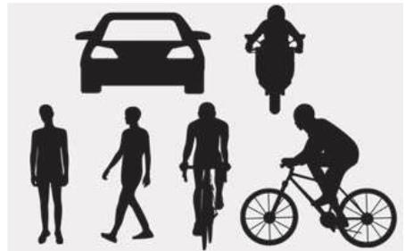
The illustration above shows the image the front view camera is capable of detecting as a vehicle, powered two-wheeler, pedestrian, or cyclist.
