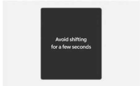
Repeated sudden acceleration and quick start may temporarily overheat the transmission. Wait until the system to cool before operating the rotary gear shift dial.
