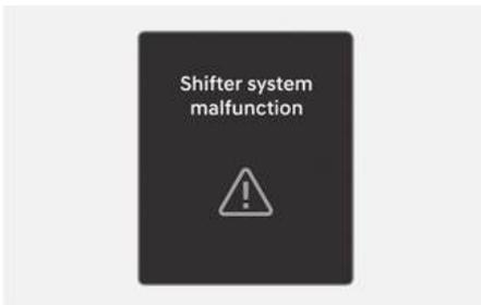
This message appears when the transmission or the shift dial does not properly operate in the P (Park) position. Have your vehicle inspected by an authorized HYUNDAI dealer.
