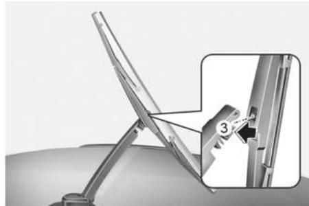
4. If the replacement is complete, put down the wiper arm onto the rear windshield, and turn the vehicle ON and operate the wipers to check the blade is installed correctly.
