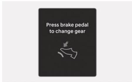
This message appears when the brake pedal is not depressed while shifting the gear.
