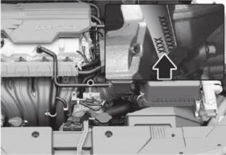
The engine number is stamped on the engine block as shown in the drawing.
