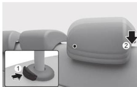
1. Put the head restraint poles into the holes (2) while pressing the release button (1).
