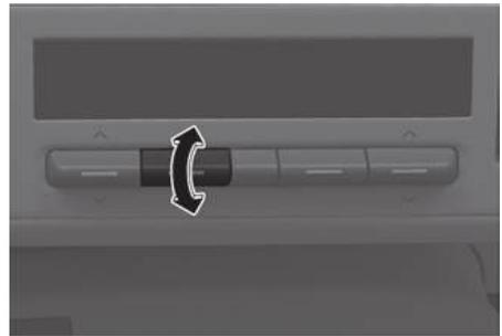
Push up the switch to increase fan speed and airflow. Push down the switch to decrease fan speed and airflow.
