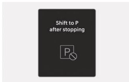
This message appears when the gear is shifted to P (Park) while the vehicle is moving.
