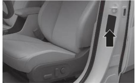
The vehicle certification label attached on the driver's (or front passenger's) side center pillar gives the Vehicle Identification Number (VIN).
