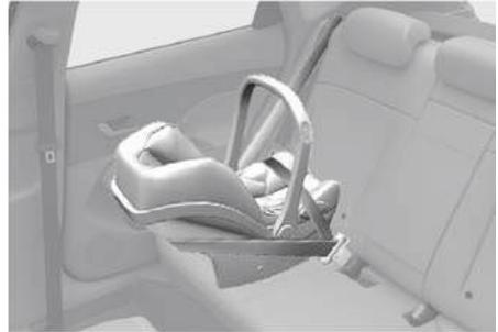
A rearward-facing Child Restraint System provides restraint with the seating surface against the back of the child. The harness system holds the child in place, and in an accident, acts to keep the child positioned in the Child Restraint Systems and reduce the stress to the fragile neck and spinal cord.
