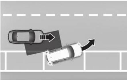
When you are driving forward out of a parking space, if Blind-Spot Collision-Avoidance Assist judges that there is a collision risk with an approaching vehicle in the blind spot, it can help avoid collision by applying the brake.
