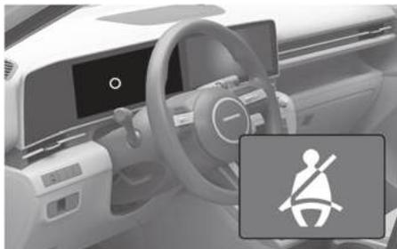
As a reminder to the driver, the driver's seat belt warning lights illuminates for about 6 seconds each time the Engine Start/Stop button is in the ON position regardless of seatbelt fastening.
