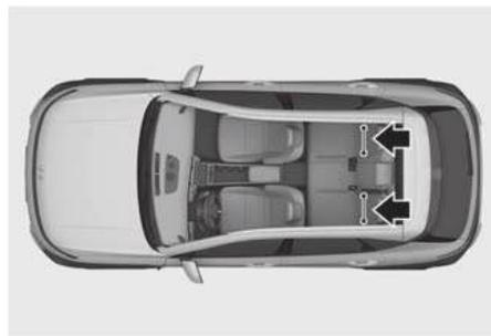
LATCH anchors have been provided in the left and right outboard rear seating positions. Their locations are shown in the illustration. There are no LATCH anchors provided for the center rear seating position.
