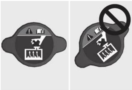
2. Make sure that the tiny protrusions inside the coolant cap is securely interlocked.
