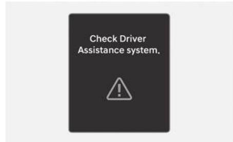
When Forward Collision-Avoidance Assist is not working properly, the "**Check Driver Assistance system.**" warning message will appear, and the
