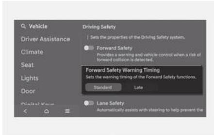
With the engine on, select **Setup > Vehicle > Driver Assistance > Driving Safety > Forward Safety Warning Timing** settings menu in the infotainment system to change the initial warning activation time for Forward Collision-Avoidance Assist. The warning time can be set to either **Standard** or **Late**
