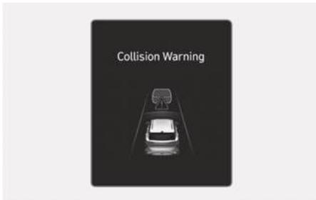
To warn the driver of a collision, the "**Collision Warning**" warning message appears and the (⚠️) warning light blinks on the instrument cluster with a warning sound and the steering wheel vibrates.
