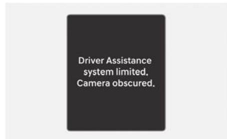
When the front windshield where the front view camera is located or the sensor is covered with foreign material, such as snow or rain, or when severe weather conditions are present such as fog or heavy rainfall, it can reduce the detecting performance and temporarily limit or disable Forward Collision-Avoidance Assist.
