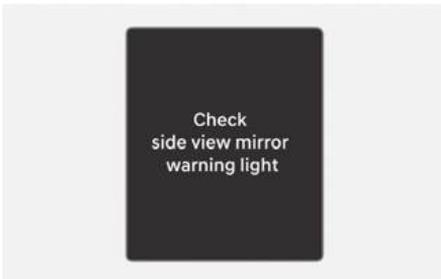
When the side view mirror warning light is not working properly, the "**Check side view mirror warning light**" warning message will appear on the instrument cluster for several seconds, and the master (⚠) warning light will appear on the instrument cluster. If this occurs, have the vehicle inspected by an authorized HYUNDAI dealer.
