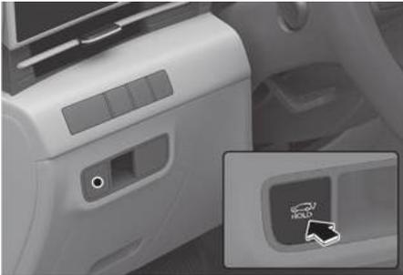
When the liftgate is closed, press the power liftgate open/close button. The power liftgate opens with a warning sound.
