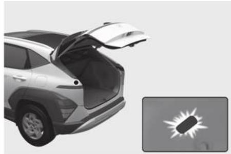
The cargo area lamp turns on when the liftgate is opened and off when the liftgate is closed.
