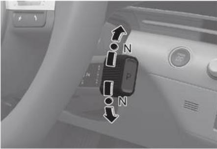
To shift the gear to N (Neutral), rotate the rotary gear shift dial to N (Neutral) from R (Reverse) or D (Drive) while depressing the brake pedal.
