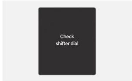
This message appears when there is a malfunction with the rotary gear shift dial. Have your vehicle inspected by an authorized HYUNDAI dealer.
