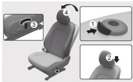
1. Recline the seat back by pressing seatback angle lever or switch (3).
