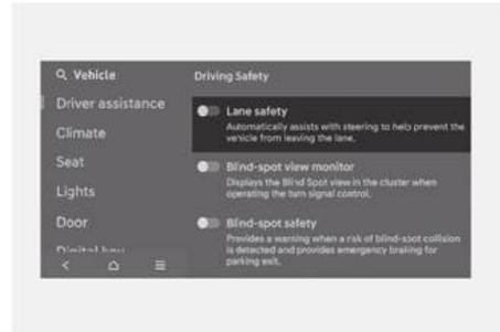
With the engine on, select **Setup > Vehicle > Driver Assistance > Driving Safety > Lane Safety** from the settings menu in the infotainment system to set whether to use each function.
