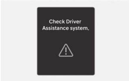
When Blind-Spot Collision Warning is not working properly, the "**Check Driver Assistance system.**" warning message will appear on the instrument cluster for several seconds, and the master (⚠) warning light will appear on the instrument cluster. If this occurs, have the vehicle inspected by an authorized HYUNDAI dealer.
