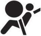
The SRS (Supplemental Restraint System) airbag warning light on the instrument panel displays the airbag symbol in the illustration. The light indicates if there is a potential problem with your airbag system, which could include your side and/or curtain airbags used for rollover protection.
