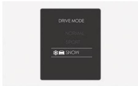
The mode changes, as the following, whenever the DRIVE MODE knob is turned to the right or left or the drive mode switch is pushed up or down.
