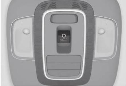
The sunroof can only be operated when the Engine Start/Stop button is in the ON or START position.
