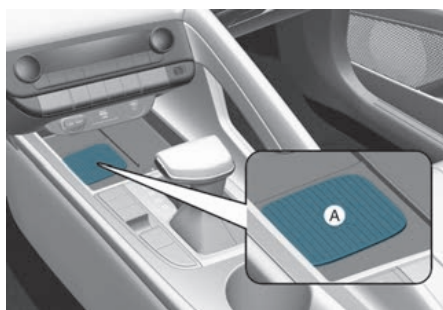
[A] Vehicle authentication pad (Wireless charging pad)
