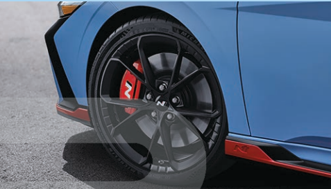
19” forged wheels and 14.2” front brake rotors
