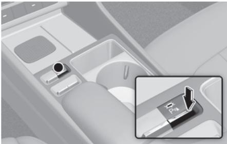
Press the Parking Safety (P<sub>W</sub>) button to turn on Parking Distance Warning. Press the button again to turn off the function.
