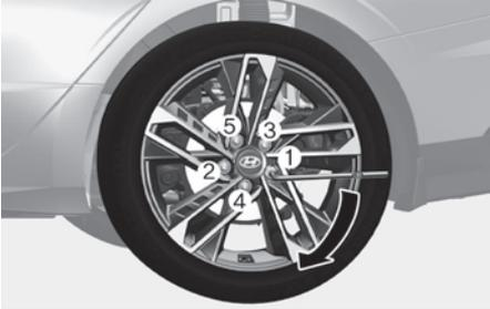
Check the tire pressure after installing the compact spare tire. The compact spare tire should be inflated to 60 psi (420 kPa). If you have a tire gauge, check the tire pressure (refer to the "Tires And Wheels" section in chapter 2 for tire pressure instructions). If the spare tire pressure is lower or higher than the recommended, drive slowly to the nearest service station and adjust it to the recommended pressure.
