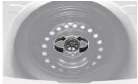
Turn the winged hold down bolt counterclockwise to remove the spare tire.
