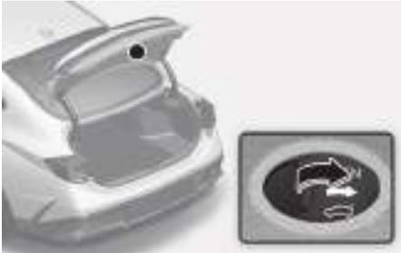
Your vehicle is equipped with the emergency trunk safety release lever located on the bottom of the trunk. When someone is inadvertently locked in the trunk, the trunk can be opened by moving the lever in the direction of the arrow and pushing the trunk open.
