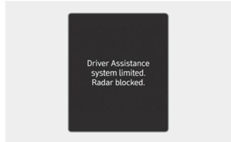
When the rear bumper around the rear corner radar or sensor is covered with foreign material, such as snow or rain, or installing a trailer or carrier, it can reduce the detecting performance and temporarily limit or disable Safe Exit Warning.
