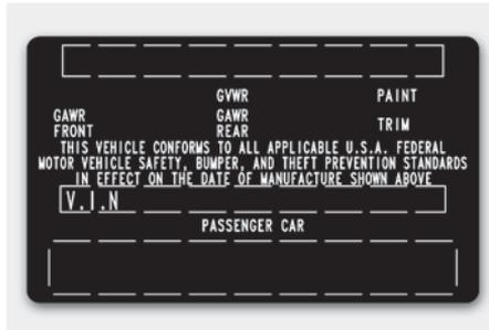
The certification label is located on the driver's door sill at the center pillar and shows the maximum allowable weight of the fully loaded vehicle. This is called the GVWR (Gross Vehicle Weight Rating). The GVWR includes the weight of the vehicle, all occupants, fuel and cargo. This label also tells you the maximum weight that can be supported by the front and rear axles, called Gross Axle Weight Rating (GAWR).
