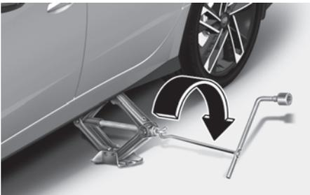
9. Loosen the wheel nuts with the wheel lug wrench and remove them with your fingers. Remove the wheel from the studs and lay it flat on the ground out of the way. Remove any dirt or debris from the studs, mounting surfaces, and spare tire.
