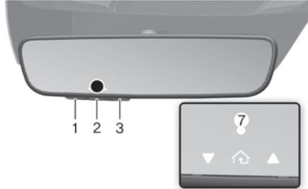
1. Press and release the HomeLink button (1), (2) or (3), you would like to program. The HomeLink indicator light (7) will flash orange slowly (if not, perform the steps of "Erasing HomeLink Buttons" section, and start over).
