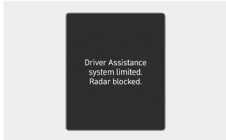
When the rear bumper around the rear-side radar or sensor is covered with foreign material, such as snow or rain, or installing a trailer or carrier, it can reduce the detecting performance and temporarily limit or disable Rear Cross-Traffic Collision-Avoidance Assist.
