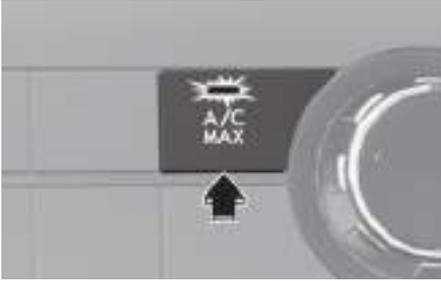
The MAX A/C mode is used to cool the inside of the vehicle faster. Air flow is directed toward the upper body and face. The air conditioning and recirculated air are both selected. Turn the fan speed mode to adjust.
