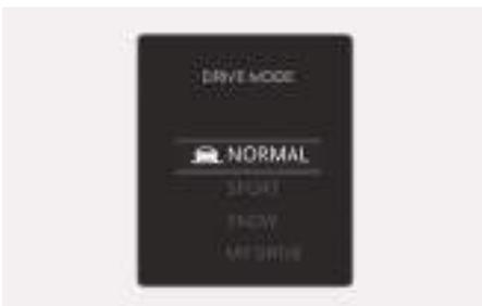
The mode changes, as the following, whenever the DRIVE MODE switch is pushed up or down.
