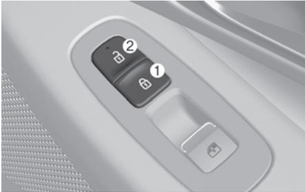
When pressing the
