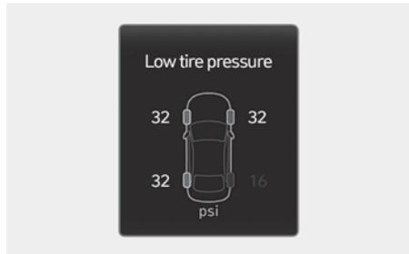
When the Tire Pressure Monitoring System warning indicator (⚠️) is illuminated and a warning message appears on the cluster display, one or more of your tires is significantly under-inflated. The Low Tire Pressure Position Telltale will indicate which tire is significantly under inflated by illuminating the corresponding parking light.
