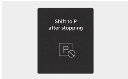
This message appears when the gear is shifted to P (Park) while the vehicle is moving.
