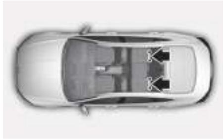
LATCH anchors have been provided in the left and right outboard rear seating positions. Their locations are shown in the illustration. There are no LATCH anchors provided for the center rear seating position.
