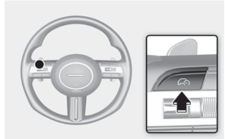
To turn Smart Cruise Control off, press the **|||** switch or the Driving Assist (DA) button.
