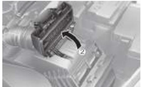
3. Rotate the fixed lever (3) on the filter and loosen the lock.
