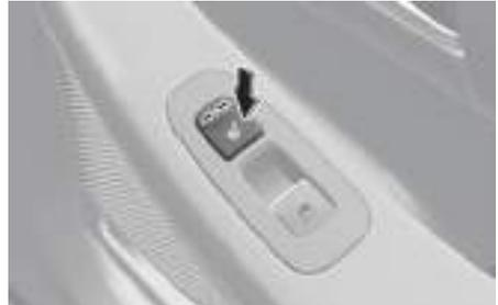
While the engine is running, press the seat warmer switch to warm the rear seats.
