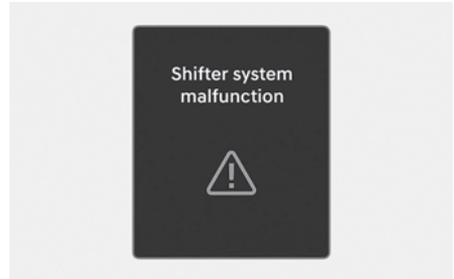
This message appears when the transmission or the shift dial does not properly operate in the P (Park) position.
