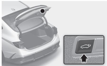
Press the power trunk close button. The trunk will close automatically.
