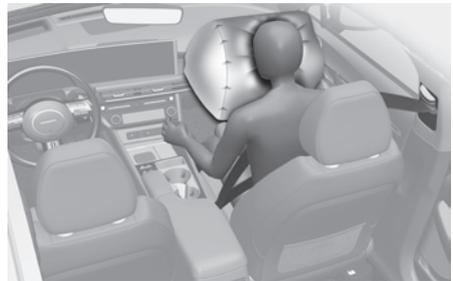
After complete inflation, the airbag immediately starts deflating, enabling the driver to maintain forward visibility and steer or operate other controls.
