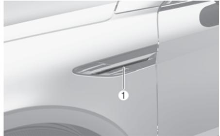
If the side repeater light (1) does not operate, have the system inspected by an authorized HYUNDAI dealer.
