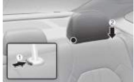
3. Route the seat belt webbing to the outward of the rear seat to prevent the belts from being damaged.
