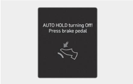
When the conversion from Auto Hold to EPB is not working properly a warning will sound and a message will appear.
