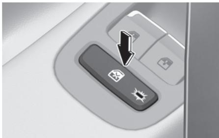
The driver can disable the power window switches on the rear passenger doors by pressing the power window lock button. When the power window lock button is pressed:
