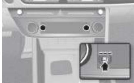
2. When you press the button, it is in the high, and you can move it in the order of medium, low, and off by pressing the button.
