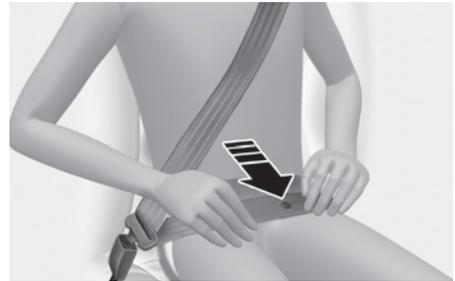
The seat belt automatically adjusts to the proper length after the lap belt portion is adjusted manually so that it fits snugly around your hips. If you lean forward in a slow, easy motion, the belt extends and moves with you.
