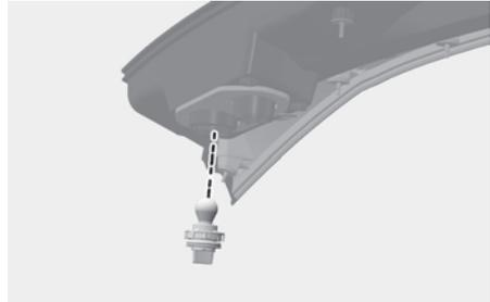
5. Remove the bulb from the socket by pressing it in and rotating it counterclockwise until the tabs on the bulb align with the slots in the socket. Pull the bulb out of the socket.
