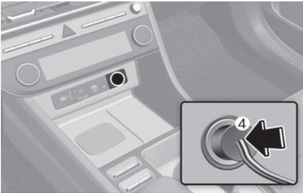
7. With the engine ON, switch on the compressor and let it run for about 5-7 minutes to fill the sealant up to proper pressure. (refer to the "Tires And Wheels" section in chapter 2). The inflation pressure of the tire after filling is unimportant and can be checked/corrected later.
