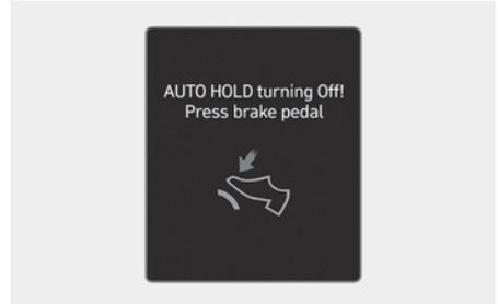
When the conversion from Auto Hold to EPB is not working properly, a warning sounds and a message appears.
