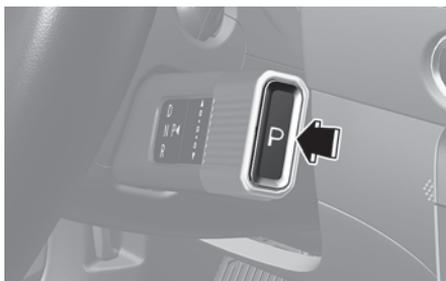
To shift the gear to P (Park), press the P button while depressing the brake pedal. If you turn the engine off in R (Reverse), N (Neutral) or D (Drive), the gear automatically shifts to P (Park).
