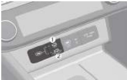
Press the USB port selection button while the engine is running. Press the upper portion of the button (1) to charge an electronic device. Press the lower portion of the button (2) to charge and listen to music with a media storage device. The USB port can be used after either indicator light turns on.
