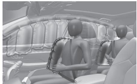
Side airbags are located in each front seat and outboard rear seats.
