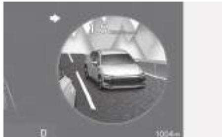
Blind-Spot View Monitor uses the wide-side view cameras to display the rear blind spot areas of your vehicle on the instrument cluster when the turn signal is turned on to help with safe lane changes.
