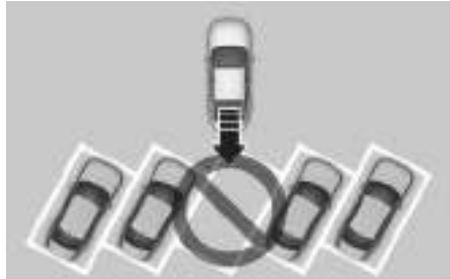
Remote Operation may not operate provide properly in a diagonal parking space.
