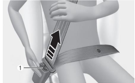
Press the release button (1) in the locking buckle.
