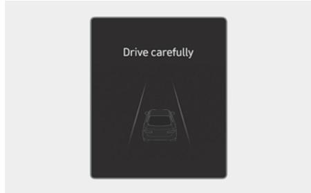
When the vehicle is stopped due to emergency braking, the "**Drive carefully**" warning message will appear on the instrument cluster.
