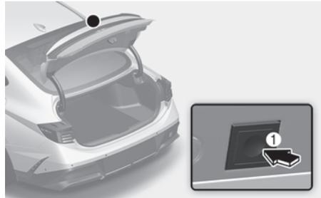
When the trunk is closed, press the power trunk open/close button to open the trunk.
