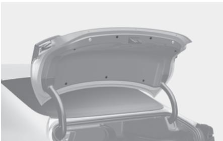
3. Remove the clip on the trunk panel.
