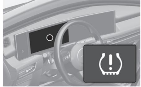
The TPMS Malfunction Indicator (
