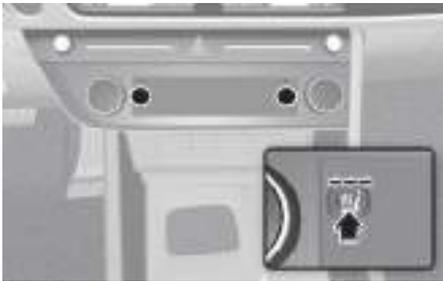
2. When you press the button, it is in the high state, and you can move it in the order of medium, low, and off by pressing the button.
