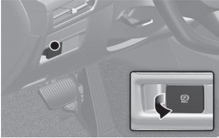
1. Depress and hold the brake pedal.
