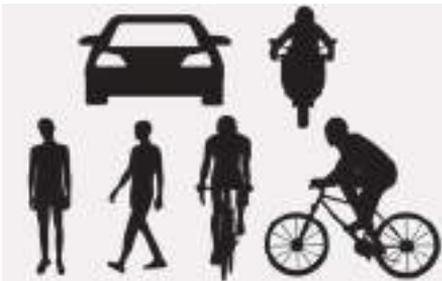
The illustration above shows the image the front view camera and front radar are capable of detecting as a vehicle, powered two-wheeler, pedestrian, or cyclist.
