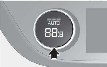
2. Turn left or right the temperature control knob to set the desired temperature. If the temperature is set to the lowest setting, the air conditioning system operates continuously. After the interior has cooled sufficiently, adjust the knob to a higher temperature set point whenever possible.
