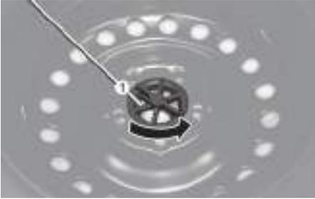
If it is hard to loosen the tire hold down wing bolt by hand, you can loosen it easily using the jack handle.
