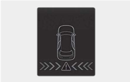
When the Rear Cross-Traffic Collision-Avoidance Assist is operating, if the function is not working normally or the radar is blocked, the master warning light (⚠) appears. You can check the warning in the Utility view on the instrument cluster.
