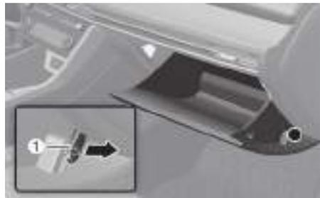
2. Press both sides of the glove box inward to release.
