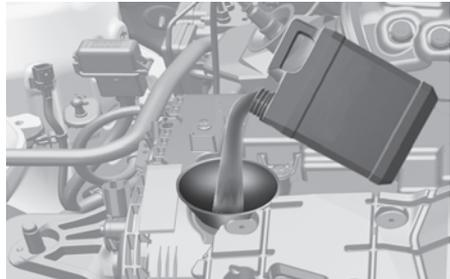
Use only the specified engine oil (Refer to the "Recommended Lubricants And Capacities" section in chapter 2).
